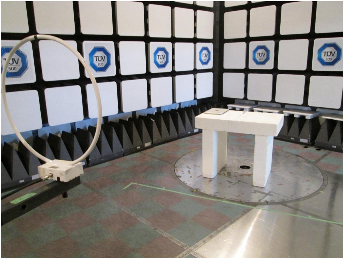
Test setup photo 1 Radiated measurements, 9 kHz – 30 MHz
