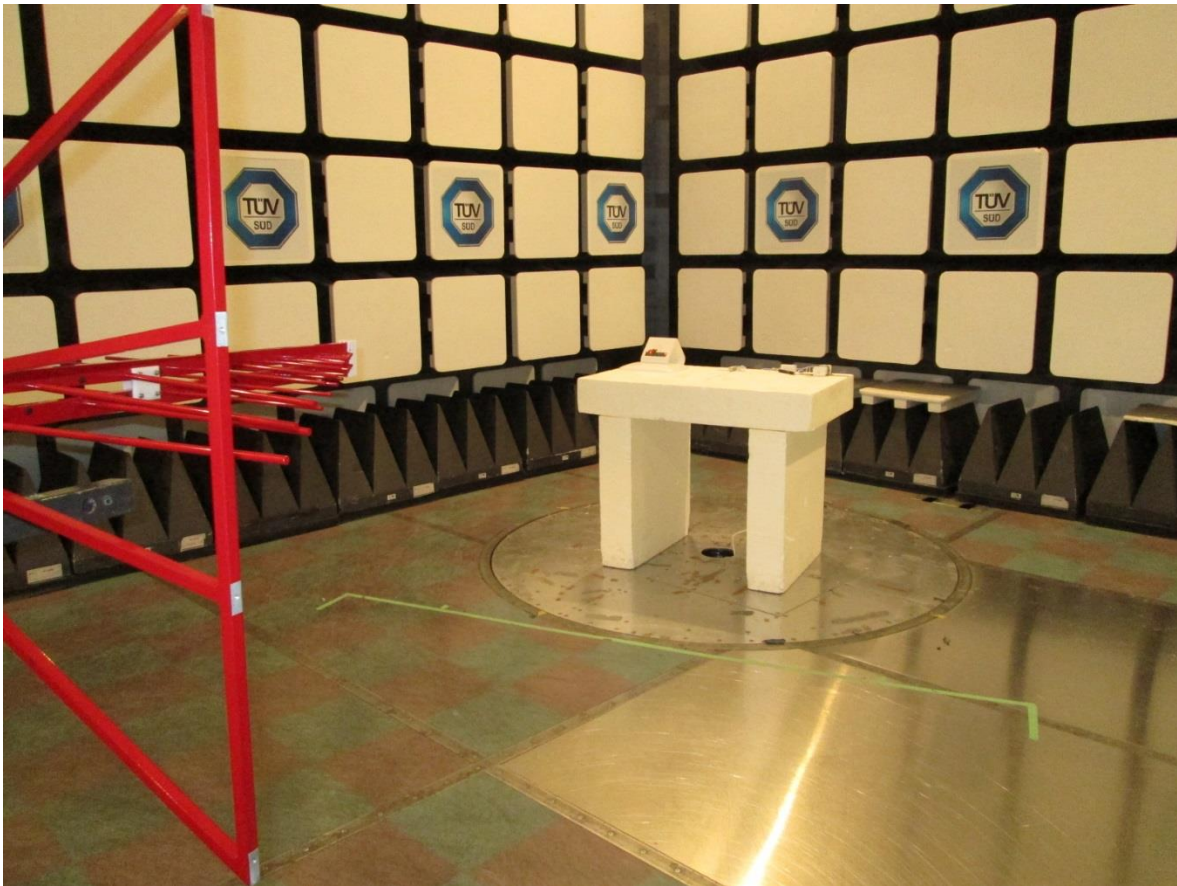
Test setup photo 2 Radiated measurements, 30 MHz – 1 GHz
