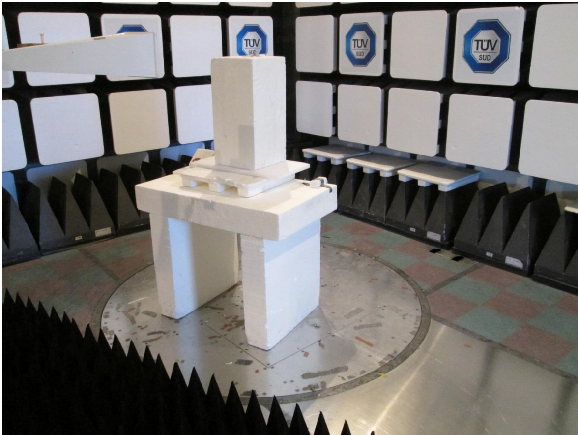
Test setup photo 5 Radiated measurements, 10 GHz – 18 GHz
