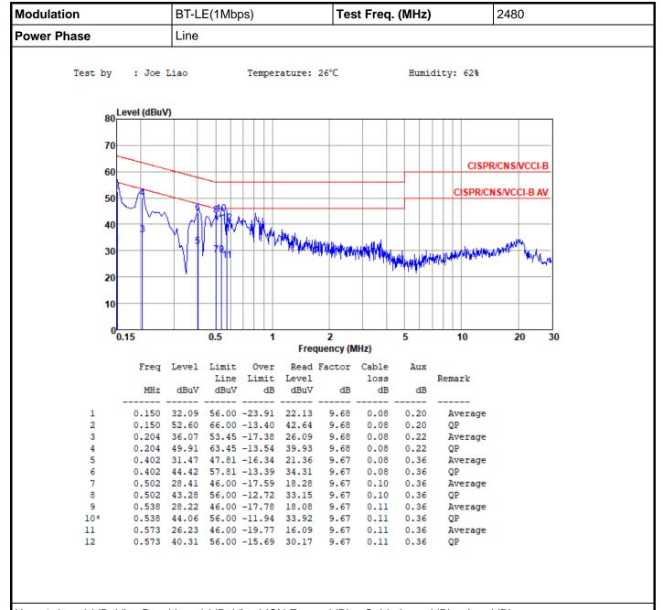
Note 1: Level (dBuV) = Read Level (dBuV) + LISN Factor (dB) + Cable Loss (dB) + Aux (dB).
