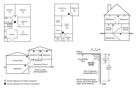
Smoke detectors should always be installed in accordance with NFPA 72, the National Fire Alarm Code. Smoke detectors should always be located in accordance with:
