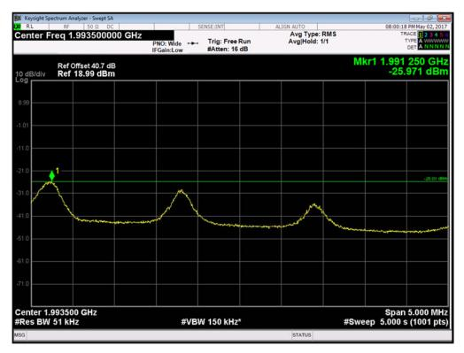
The channel power of 1MHz for 1991.250MHz is -19.44dBm, which is within the limit of -13dBm.
