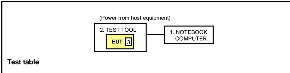
**Note:** Support unit 3 is 50ohm terminal resistor.
