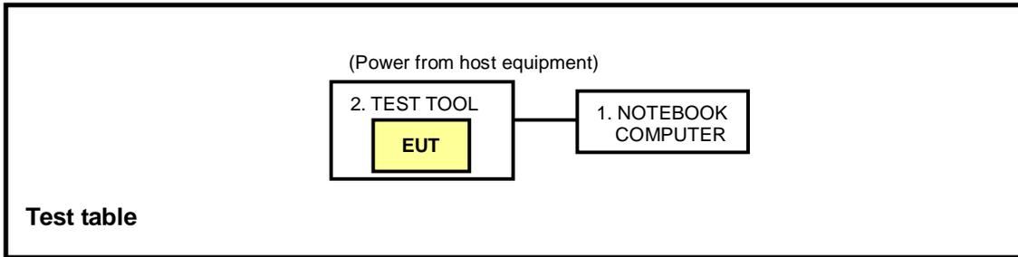
For Radiated Emission test: (above 1GHz Tx mode radiated test)
