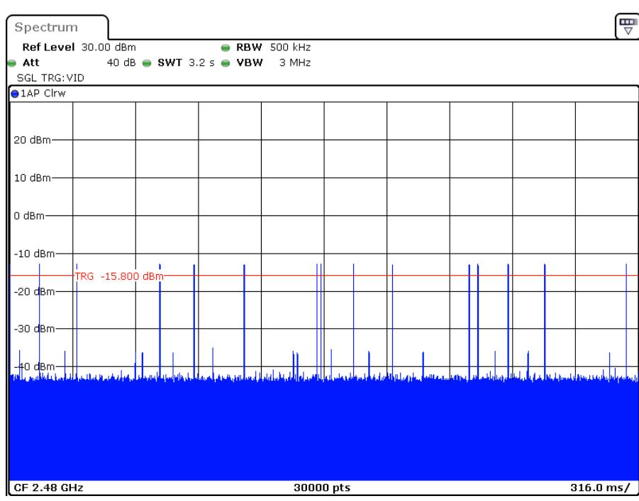
**Pulse Time, DH5, 2402 MHz**
