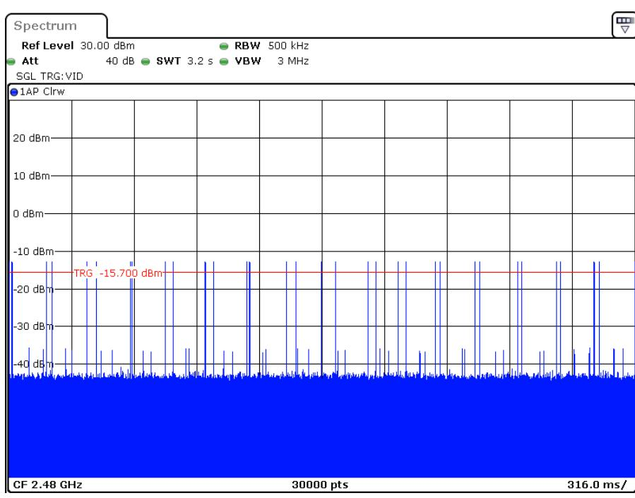
**Pulse Time, DH3, 2402 MHz**
