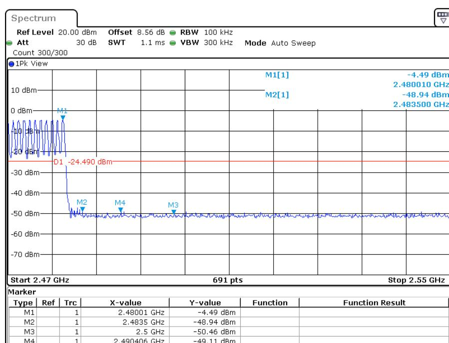
**EDR ( $\pi/4$ -DQPSK): Band Edge****Low Channel – Single**
