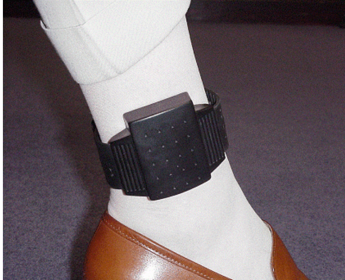
Figure 3 Protruding side of Transmitter directed upwards
