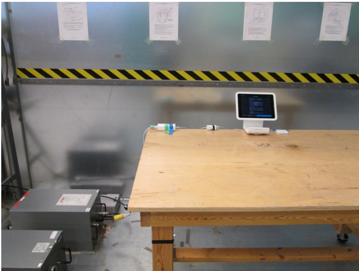
Test setup photo 3 Power line conducted emissions measurements
