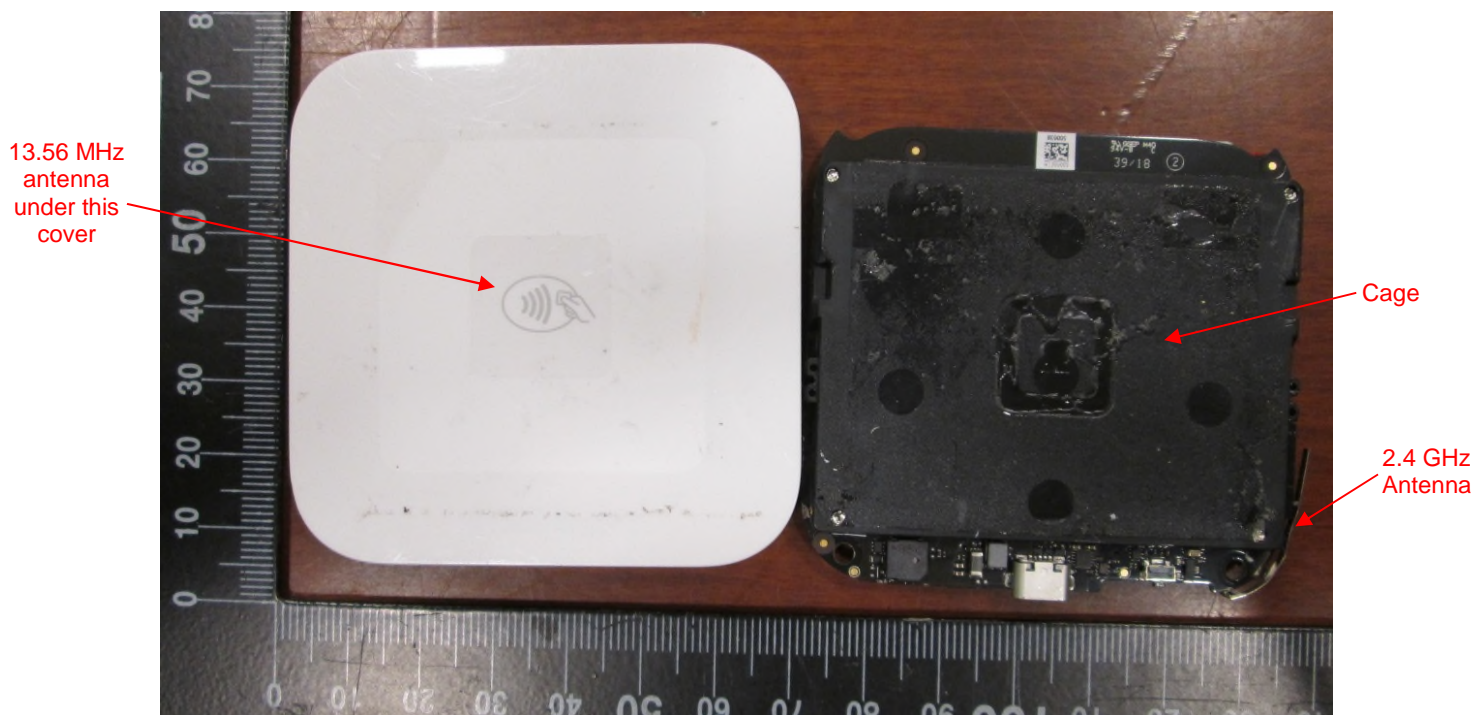
EUT – Internal view 2 PCB removed from enclosure
