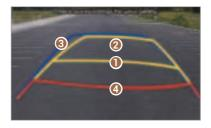
• Driving direction lines (yellow) 102 These lines show the directions of the vehicle according to the steering angle.  Neutral direction lines (blue) These lines indicate your vehicle's expected path with the steering wheel in the neutral position. It can help you determine whether the vehicle is in the correct position in a parking space and
