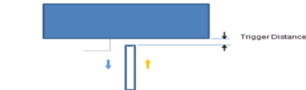
Picture: Proximity sensor triggering distances assessment (Bottom side)->
