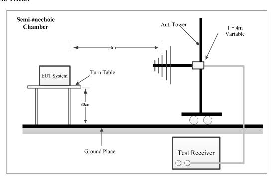
The radiated emission tests were performed in the 3 meter chamber a test site, using the setup accordance with the ANSI C63.10-2020. The specification used was the FCC Part Subpart C limits.
