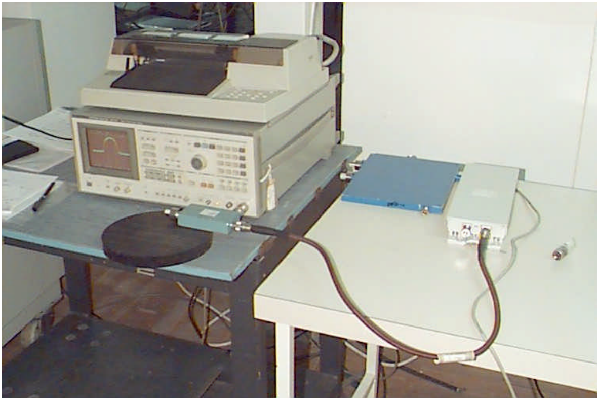
Photograph 4.1.1 Setup for minimum bandwidth measurements
