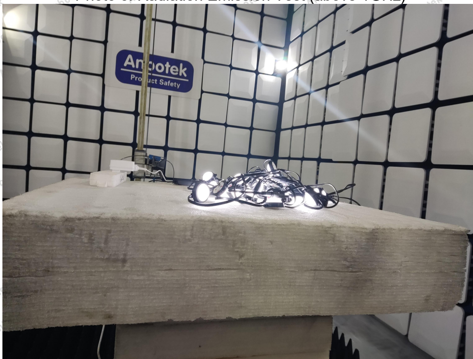
Photo of Radiation Emission Test (above 1GHz)
