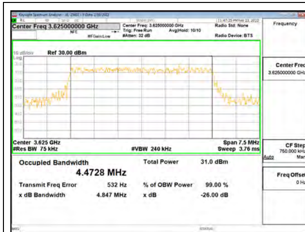
LTE B48 5MHz QPSK Middle Channel RB25-0
