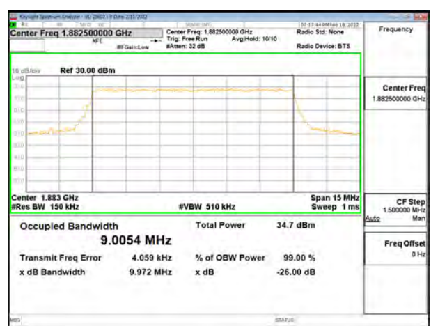
LTE B25 10MHz QPSK Middle Channel RB50-0
