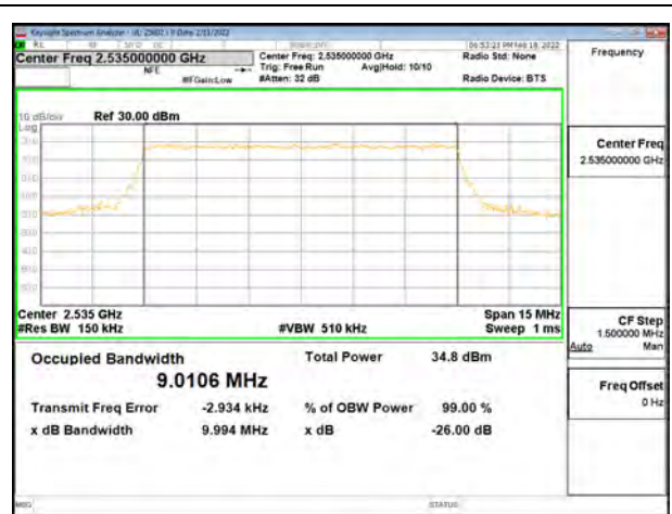
LTE B7 10MHz QPSK Middle Channel RB50-0
