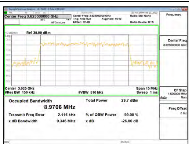
LTE B48 10MHz QPSK Middle Channel RB50-0
