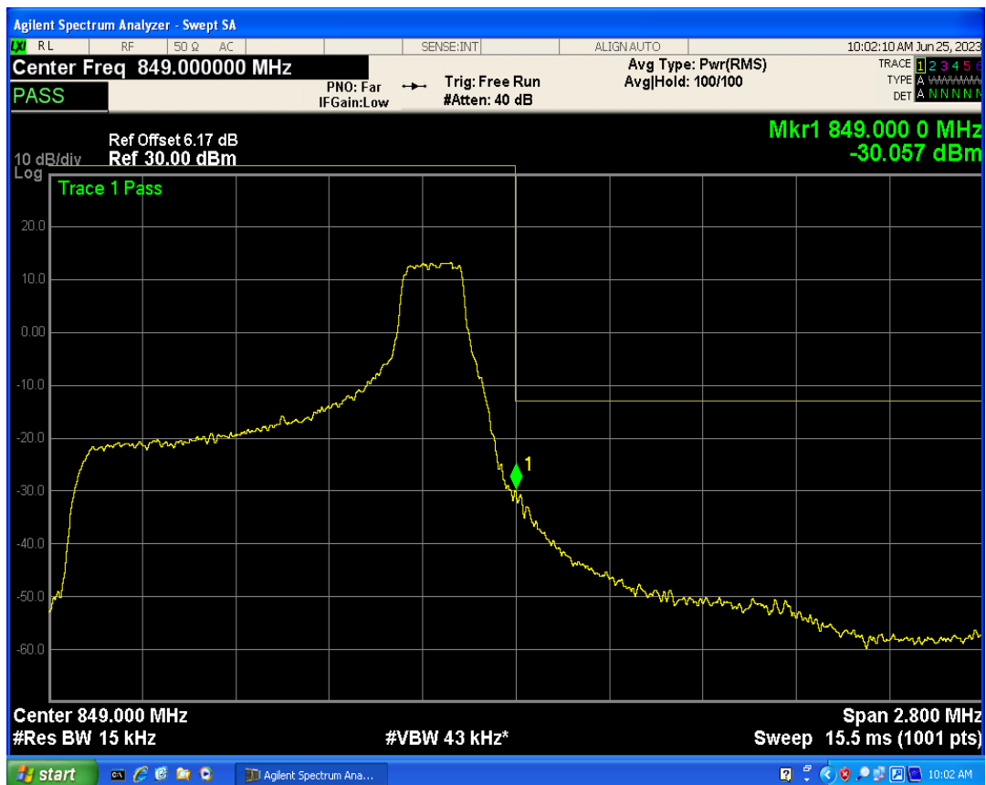
Band5 16QAM BW=1.4MHz Channel=20643 RB Size=6 Position=#0
