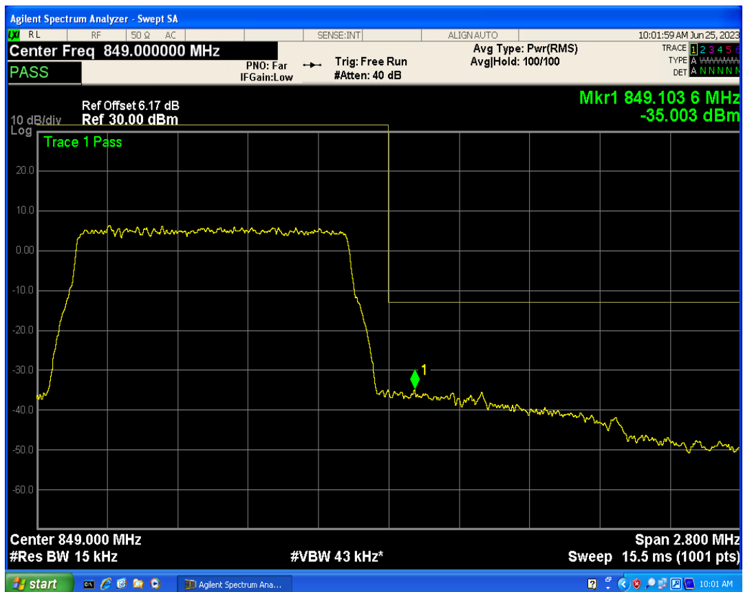
Band5 16QAM BW=1.4MHz Channel=20643 RB Size=1 Position=#0
