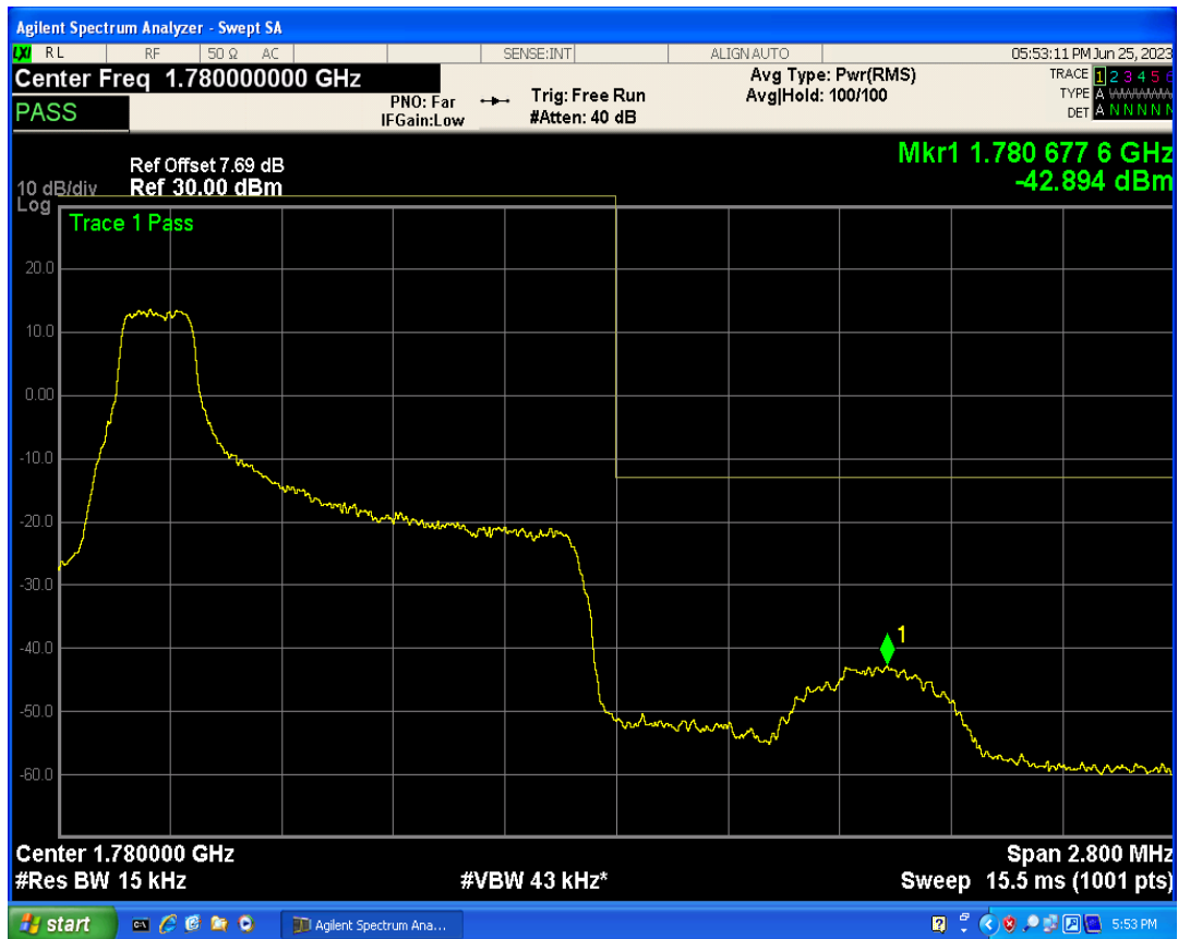
Band66 QPSK BW=1.4MHz Channel=132665 RB Size=6 Position=#0
