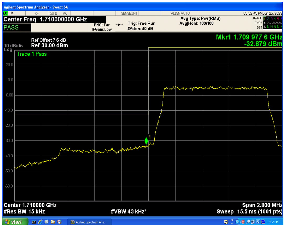
Band66 16QAM BW=1.4MHz Channel=131979 RB Size=1 Position=#0
