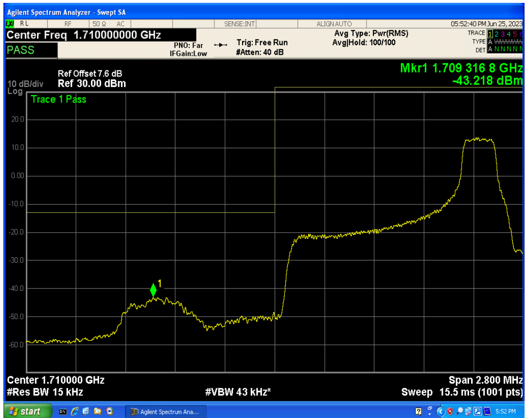
Band66 QPSK BW=1.4MHz Channel=131979 RB Size=6 Position=#0
