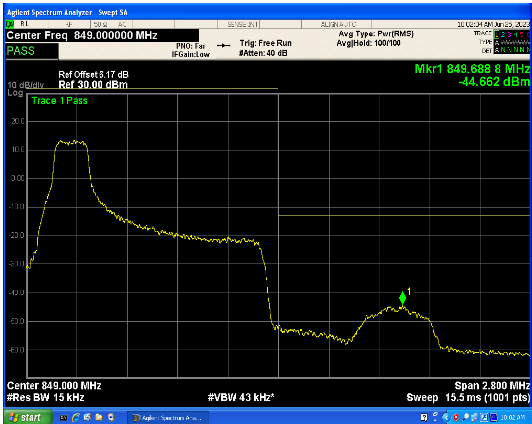
Band5 16QAM BW=1.4MHz Channel=20643 RB Size=1 Position=#Max
