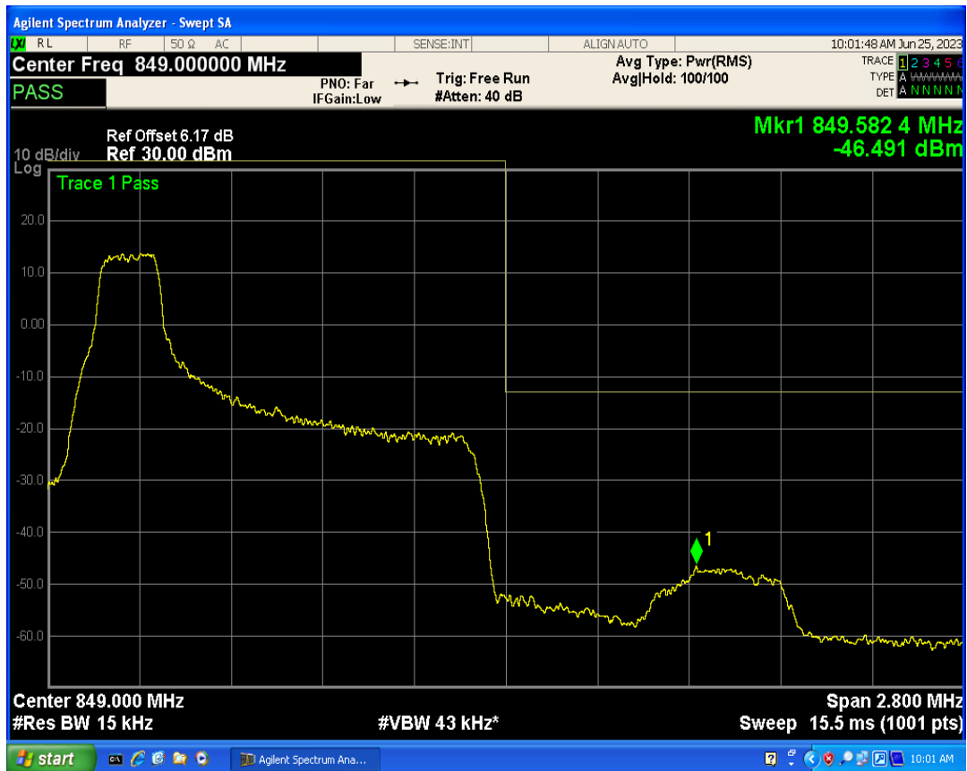
Band5 QPSK BW=1.4MHz Channel=20643 RB Size=6 Position=#0
