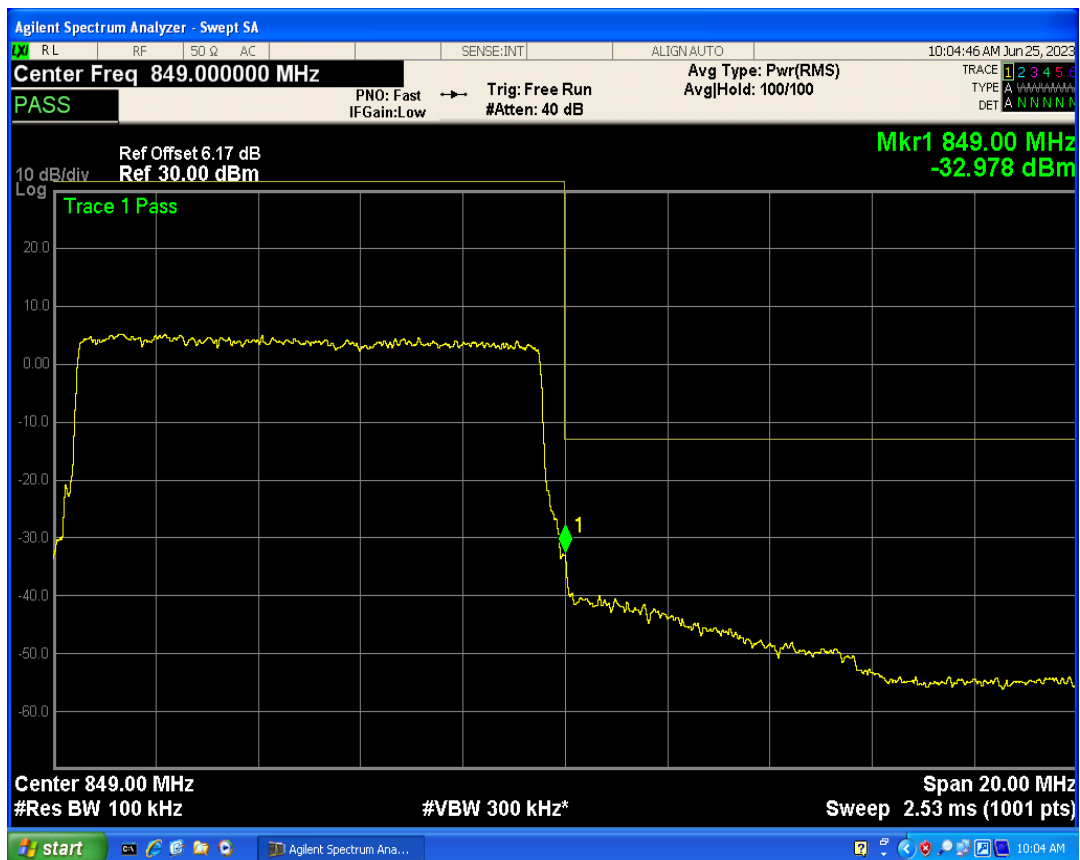
Band5 16QAM BW=10MHz Channel=20600 RB Size=1 Position=#0
