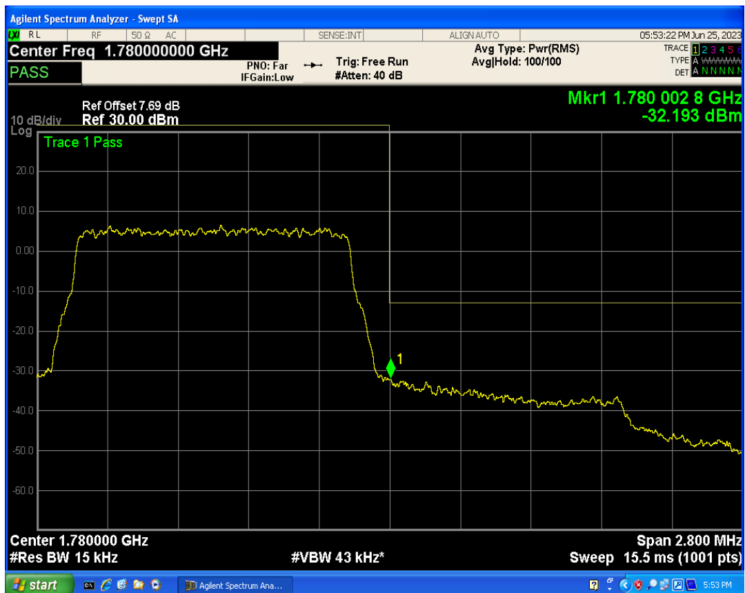
Band66 16QAM BW=1.4MHz Channel=132665 RB Size=1 Position=#0
