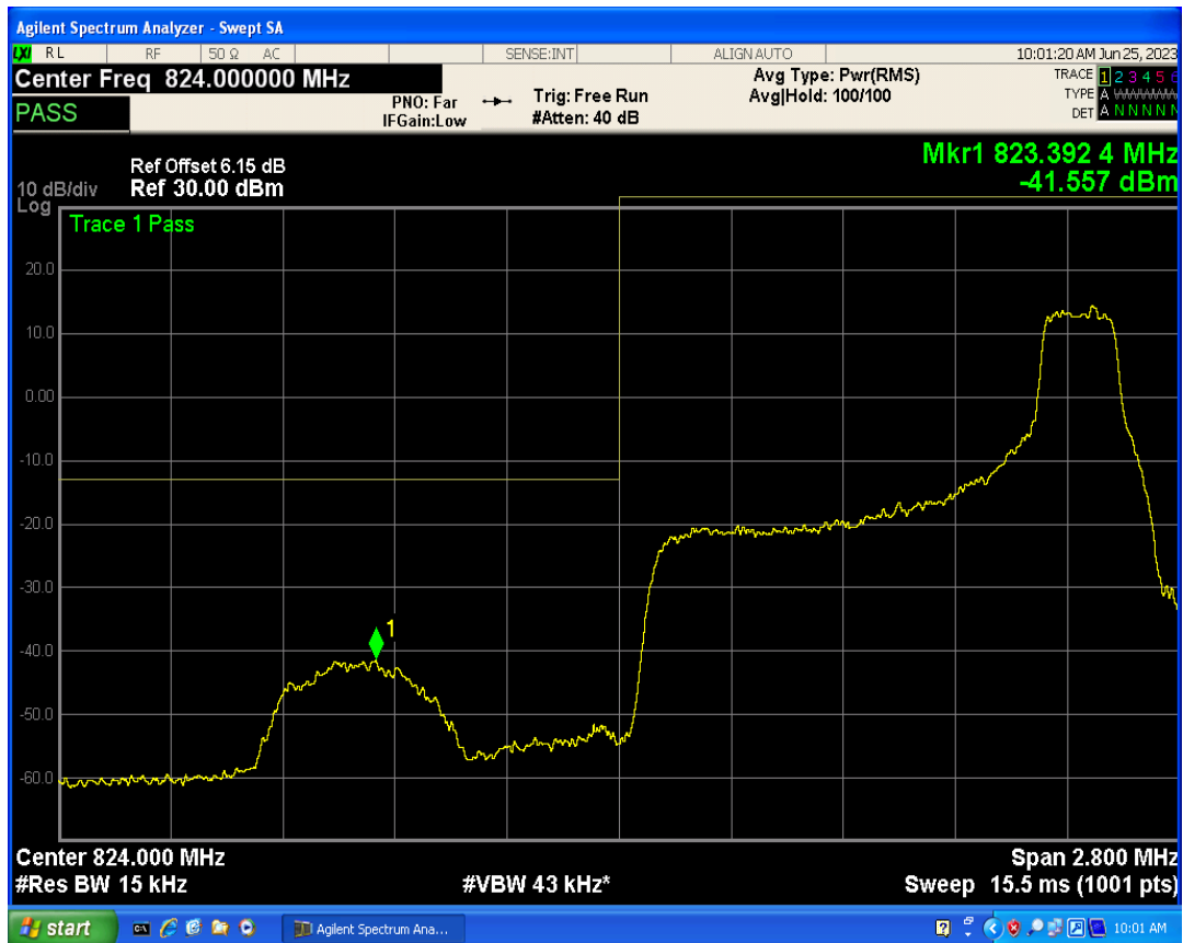
Band5 QPSK BW=1.4MHz Channel=20407 RB Size=6 Position=#0
