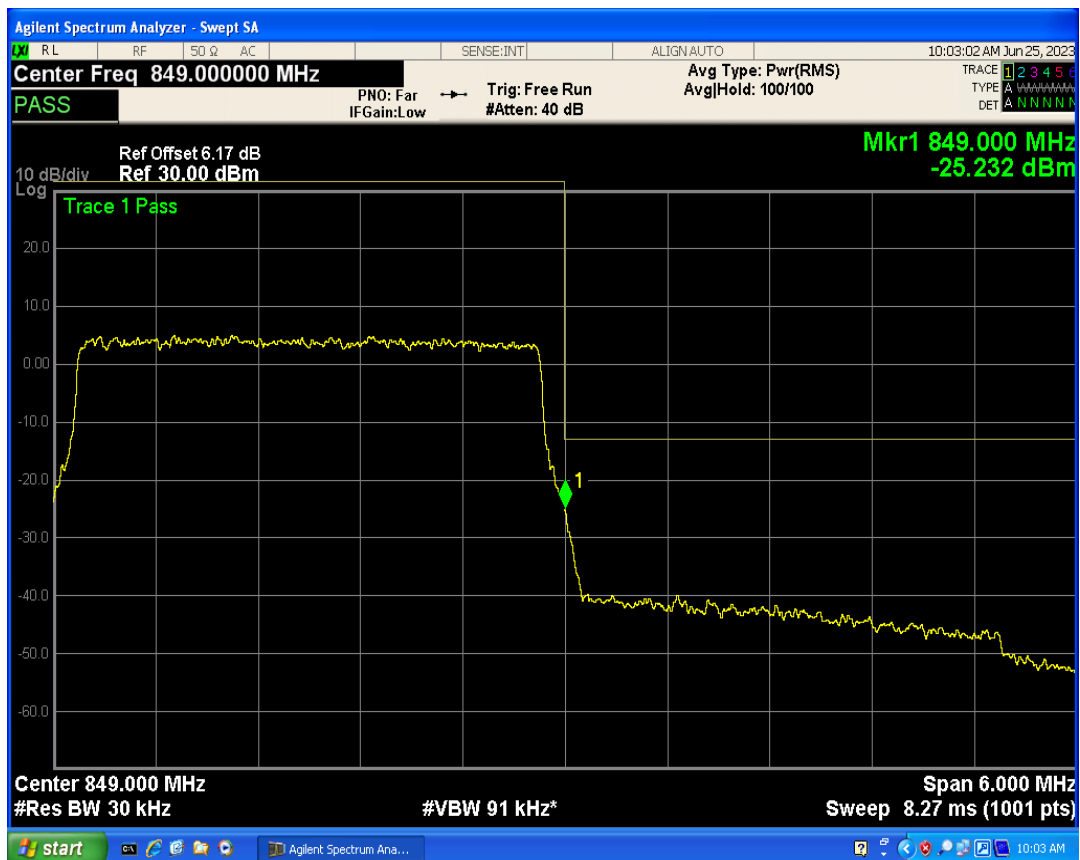
Band5 16QAM BW=3MHz Channel=20635 RB Size=1 Position=#0
