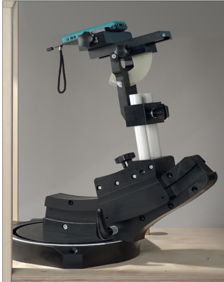
F-2. Device Holder for Transmitters
