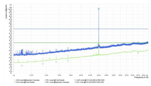
Spurious emissions from 1 GHz to 4 GHz (operation mode 4):
