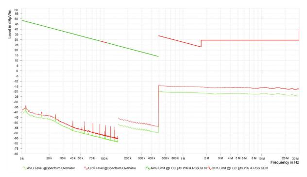
Spurious emissions from 9 kHz to 30 MHz (operation mode 4, position 2):
