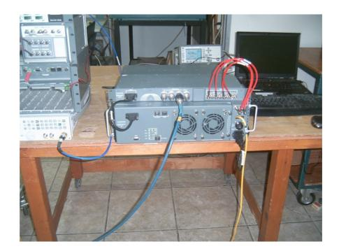
Photograph No.2 Out-of band spurious emissions measurement setup
