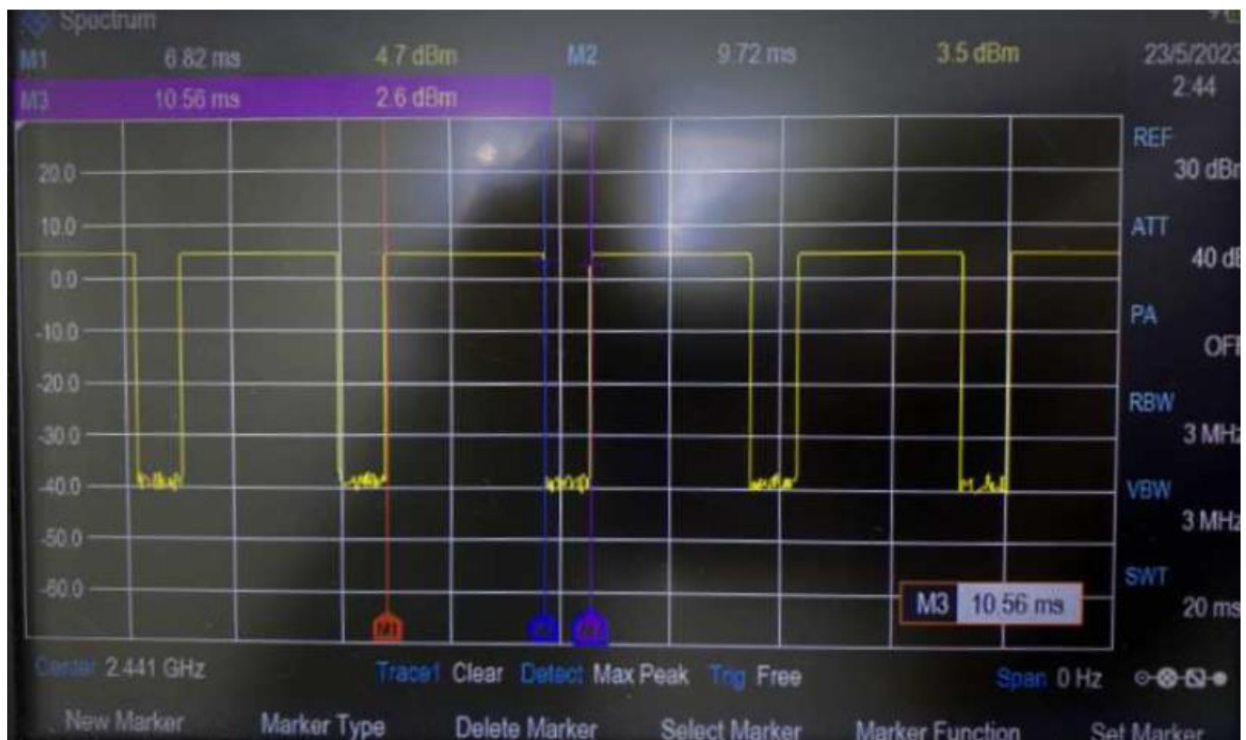
Time-domain plot for Bluetooth transmission signal
