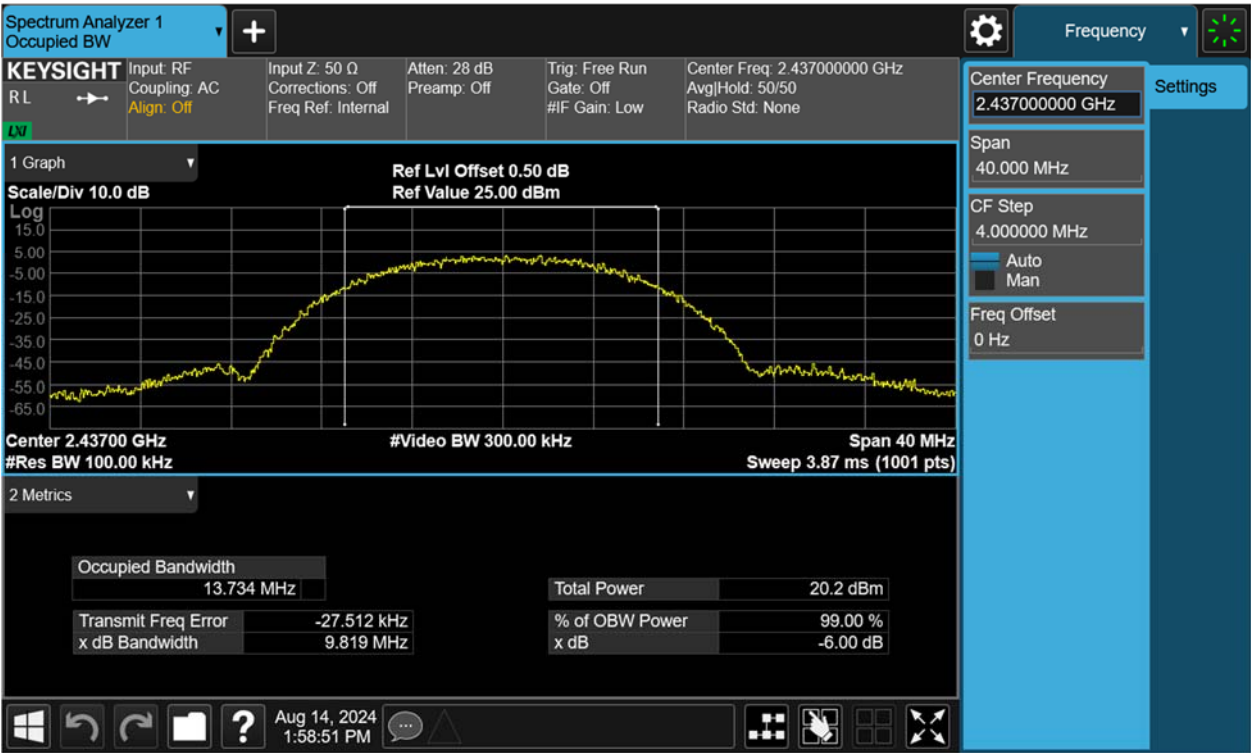
Figure 2: 6dB Bandwidth, 802.11b, 2437MHz
