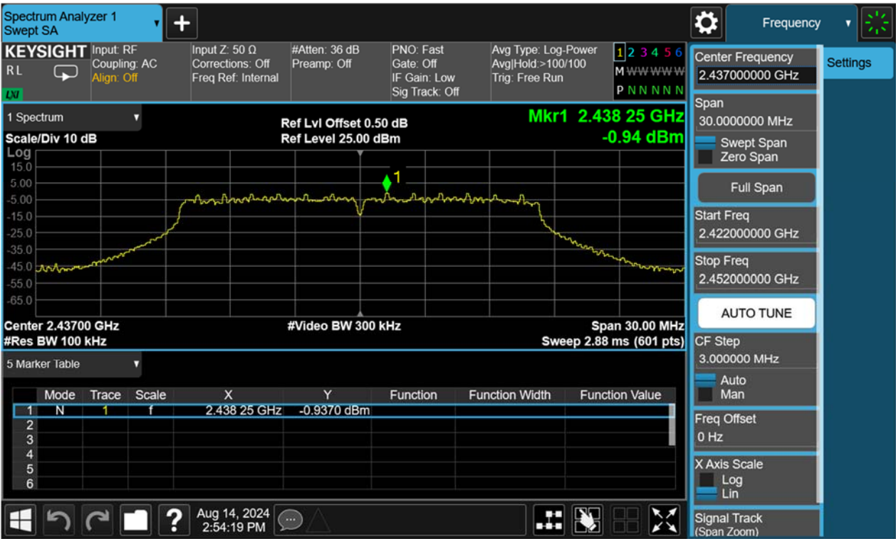
Figure 23: Conducted Spurious Emission & Authorized-band band-edge, 802.11g, 2437MHz Carrier Level
