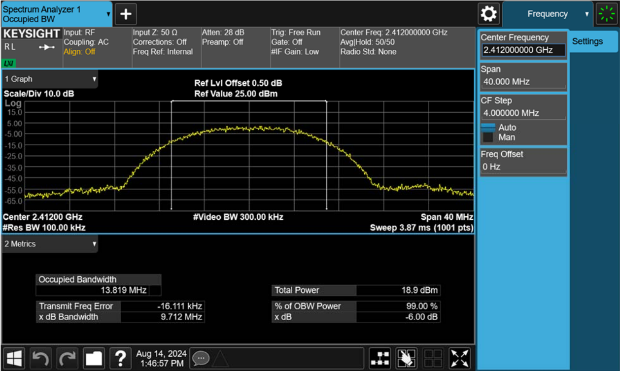
Figure 2: 6dB Bandwidth, 802.11b, 2437MHz
