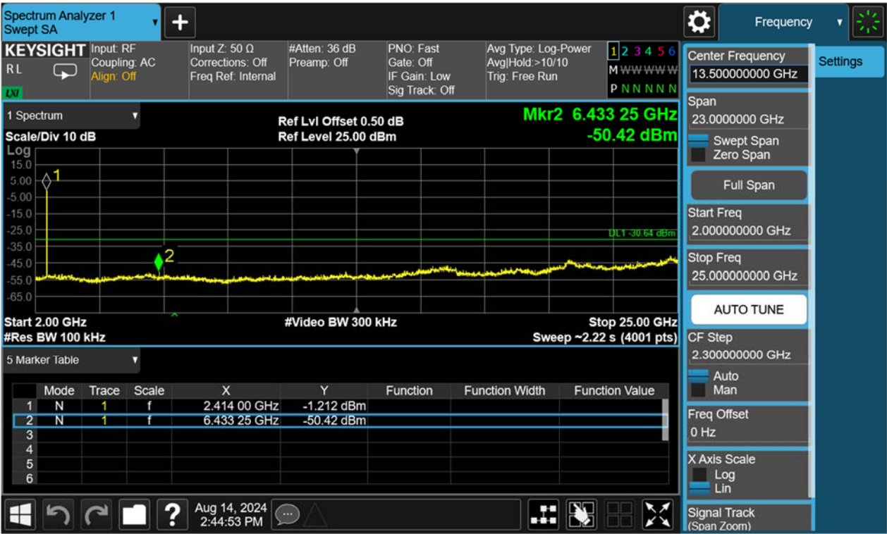
Figure 23: Conducted Spurious Emission & Authorized-band band-edge, 802.11g, 2437MHz Carrier Level
