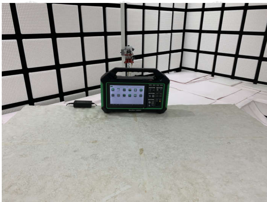
Radiated spurious emission Test Setup-2(Above 1GHz)
