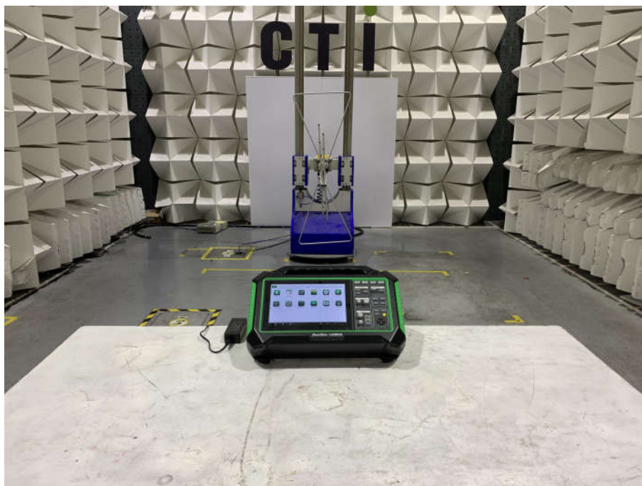
Radiated spurious emission Test Setup-1(Below 1GHz)
