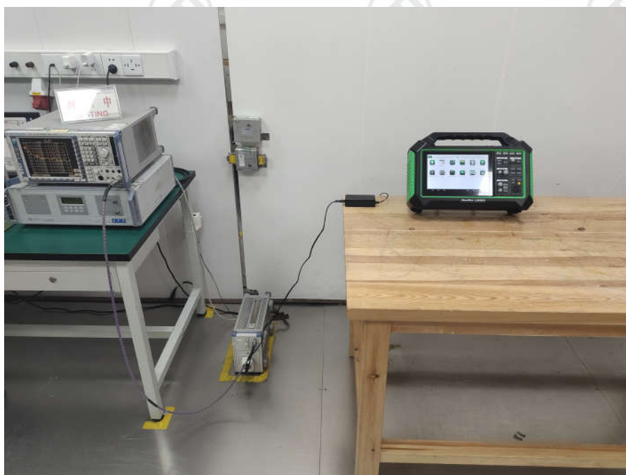
Conducted Emissions Test Setup
