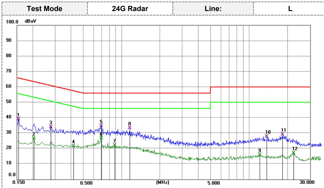
Remark: Correct Factor = Insertion loss of LISN + Cable loss + Insertion loss of Pulse Limiter;
