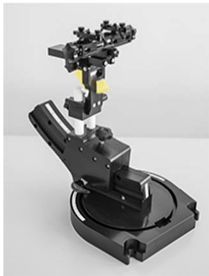
Mounting Device for Hand-Held Transmitters
