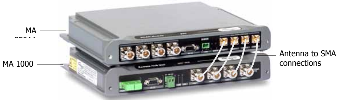
Figure 3-4. Antenna to SMA Connections
