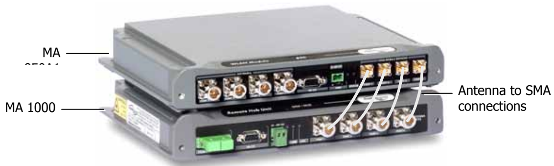
Figure 3-2. Antenna to SMA Connections
