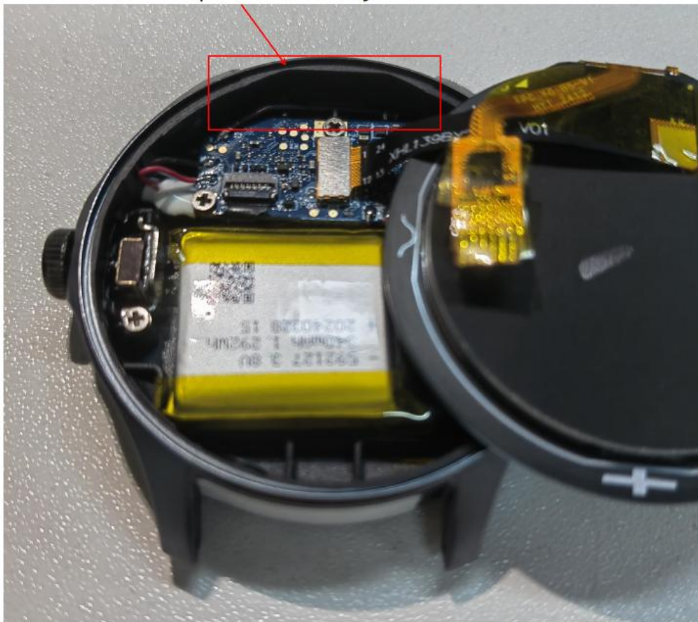
Antenna placement layout
