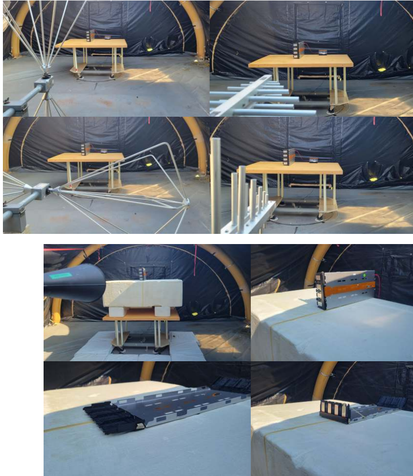
Figure 4: Radiated Emissions Test Setup Photograph(s).
