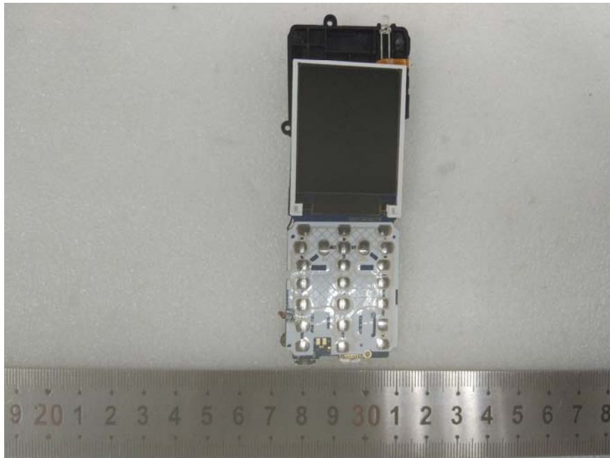
EUT – Main Board Front View
