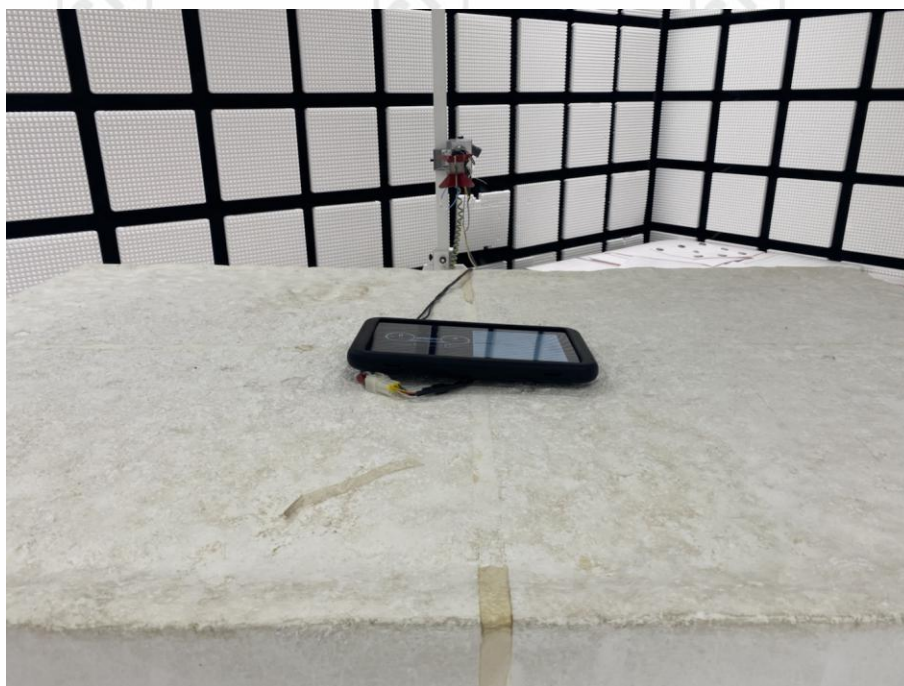
Radiated spurious emission Test Setup-2(Above 1GHz)
