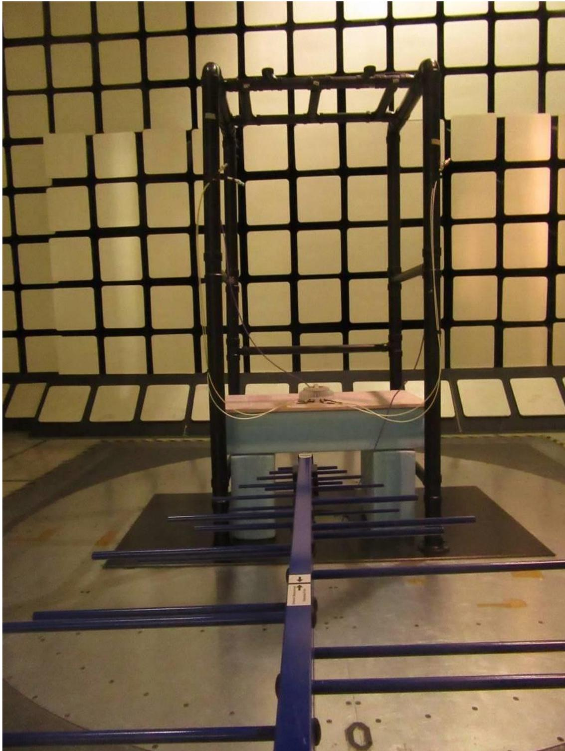
Figure 1: Radiated Test setup (30 to 1000MHz)
