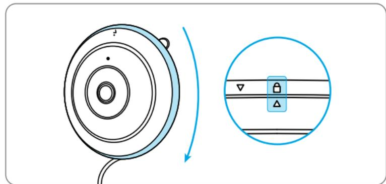
4. Attach the camera to the base and rotate the camera clockwise to lock it in position. Make sure the orientation arrow on the camera and the lock on the base are aligned.
