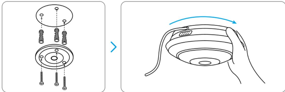
1. Drill holes in accordance with the mounting hole template. Use the drywall anchors included in the package if needed.
