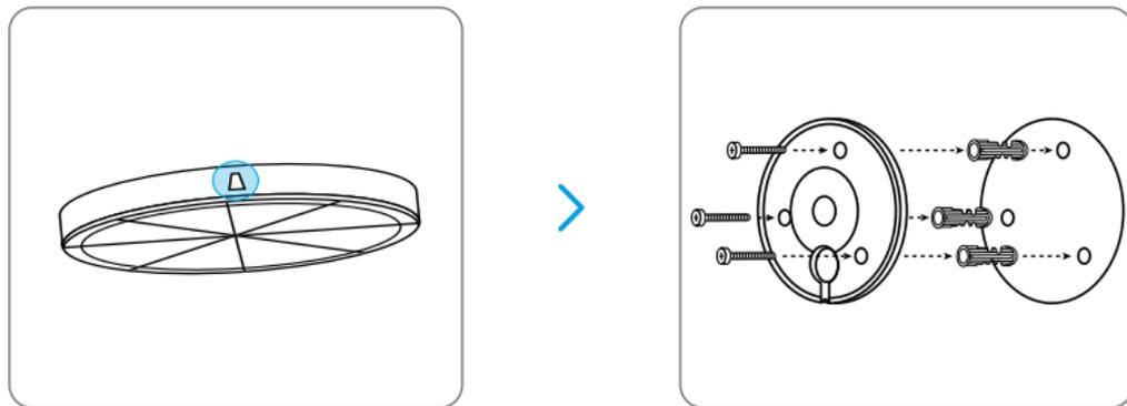
1. Before drilling the required holes, mark the direction of the lock printed on the mounting base. Make sure the lock is facing up, as shown in the diagram. This will help you align the mount base in the same orientation when installing.
