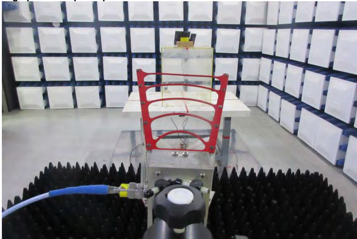
Photograph 4: Set-up for Conducted Emissions
