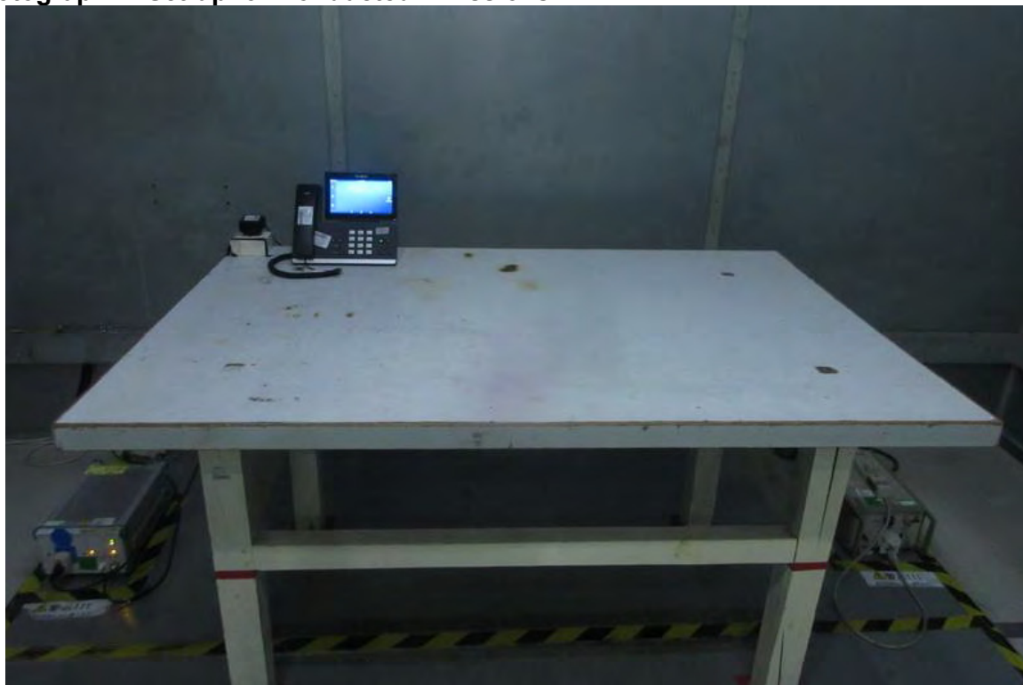
Photograph 4: Set-up for Conducted Emissions
