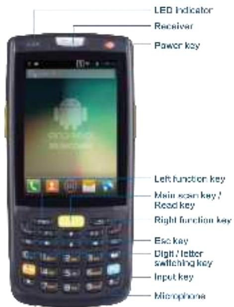
Figure 1-2 Front view of iData 95V
