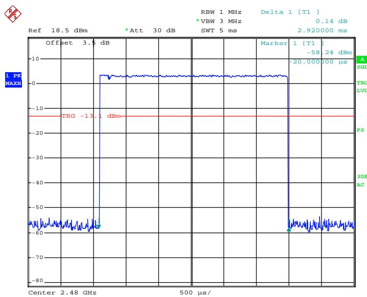
**EDR (8DPSK):****Pulse time, Low Channel, 3DH1**
