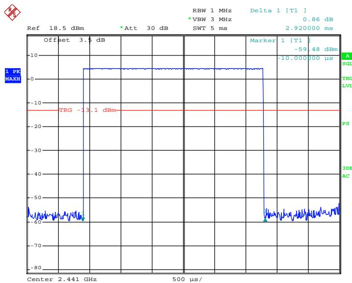
**Pulse time, High Channel, DH5**
