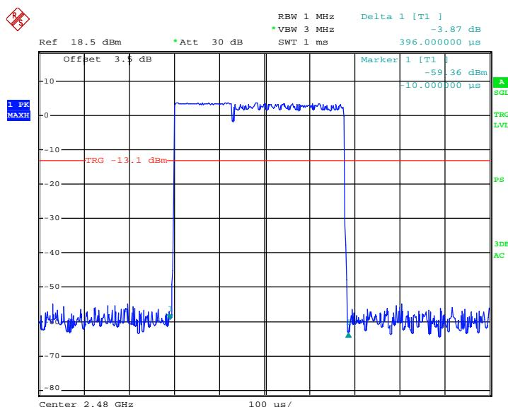
**Pulse time, Low Channel, 2DH3**
