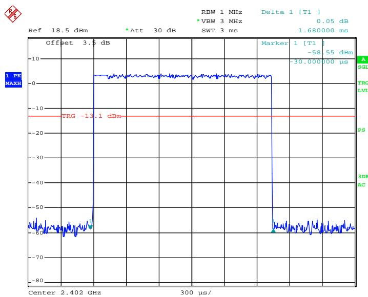
**Pulse time, Middle Channel, 3DH3**
