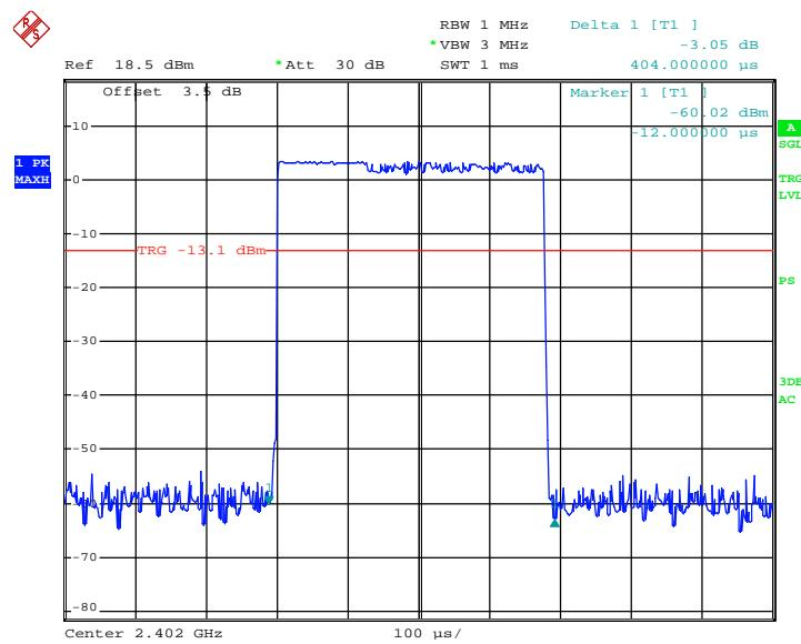
**Pulse time, Middle Channel, 2DH1**
