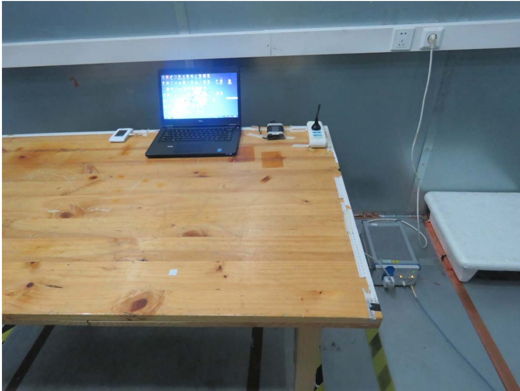
Picture 2 Conducted Emission Test Setup
