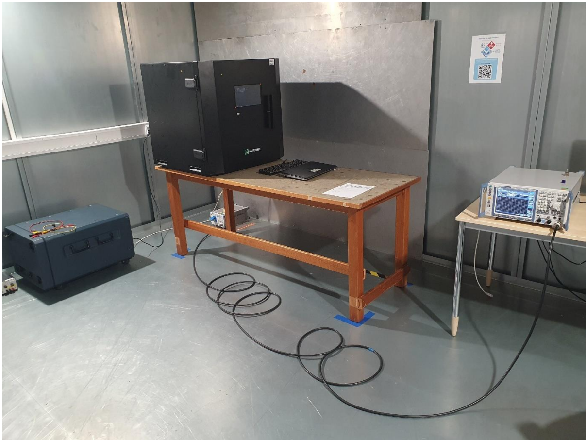
Photo 6: Photographs AC Power Line conducted emission, report section 3.3
