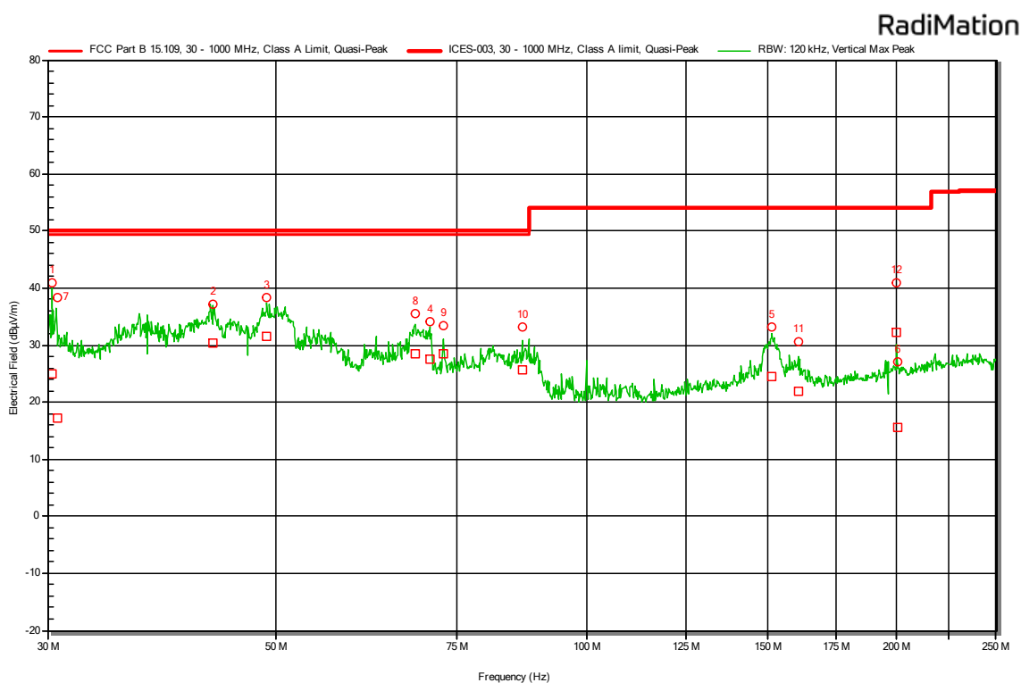
Plot 1a: radiated emissions of the EUT, Antenna vertical, in the range 30 – 250 MHz (pre-scan peak values shown)
