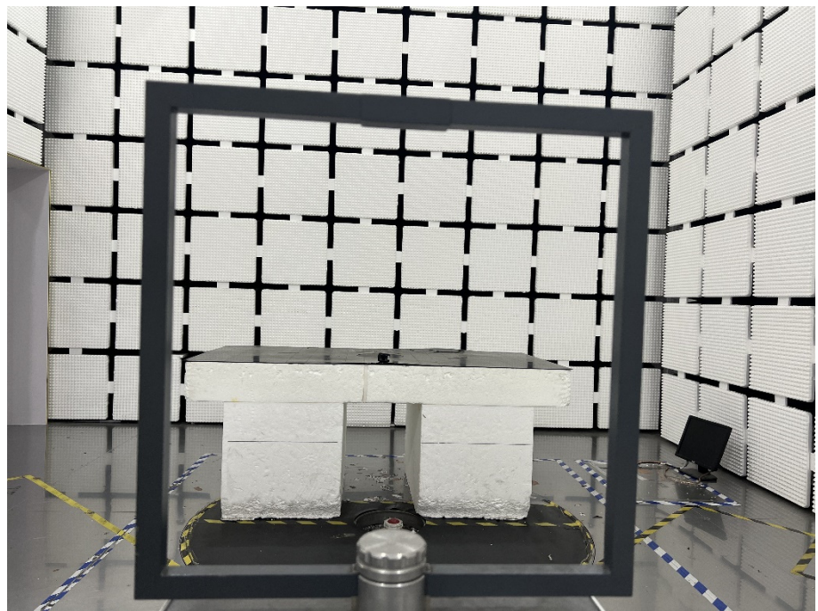
Radiation Emission Test Setup (Below 30MHz)
