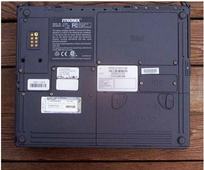
Note: Part 15.19 labeling requirement and compliance statement, located in upper left side, black label. Sample of the label text is below.
