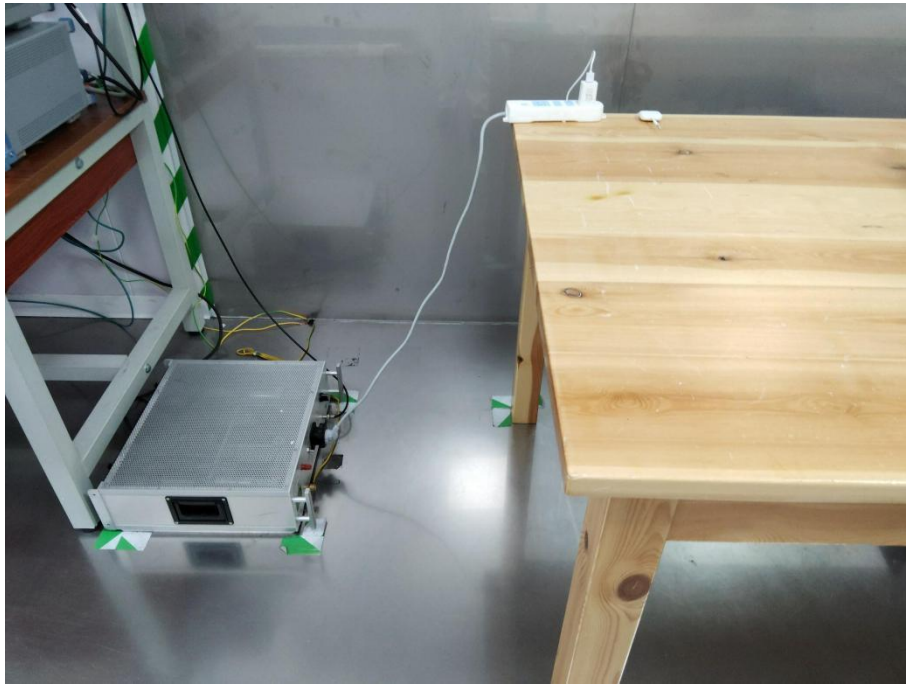
Conducted Emission at AC power line
