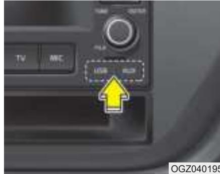
You can use an AUX port to connect audio devices and an USB port to plug in an USB or iPod®.
