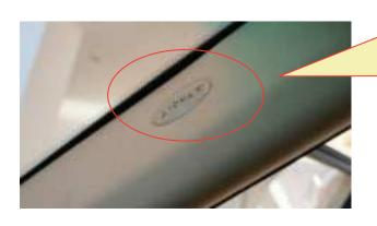
If your vehicle has side curtain airbags please be very careful when running any cables along your vehicle windows. Ensure you are not running Cable past any of the airbags as this can prevent the airbags from deploying
