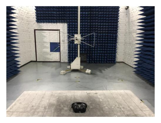
RADIATED EMISSION TEST SETUP ABOVE 1GHZ
