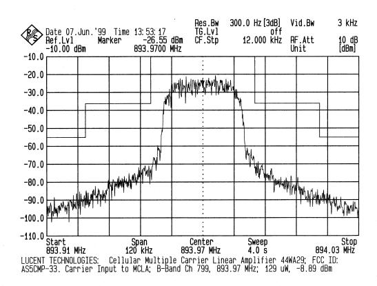
Cellular B-Band Channel 799, 893.97 MHz Cellular TDMA Multi Carrier Linear Amplifier, 44WA29, input signal to CMCLA
