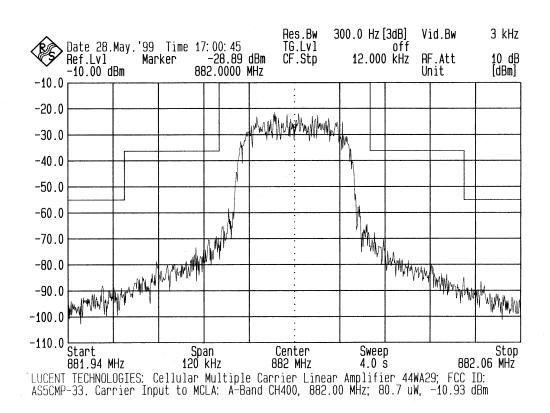
Cellular A-Band Channel 991 869.04 MHz Cellular TDMA Multi Carrier Linear Amplifier, 44WA29, input signal to CMCLA
