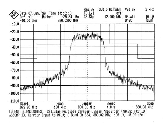
Cellular B-Band Channel 334, 880.02 MHz Cellular TDMA Multi Carrier Linear Amplifier, 44WA29, input signal to CMCLA
