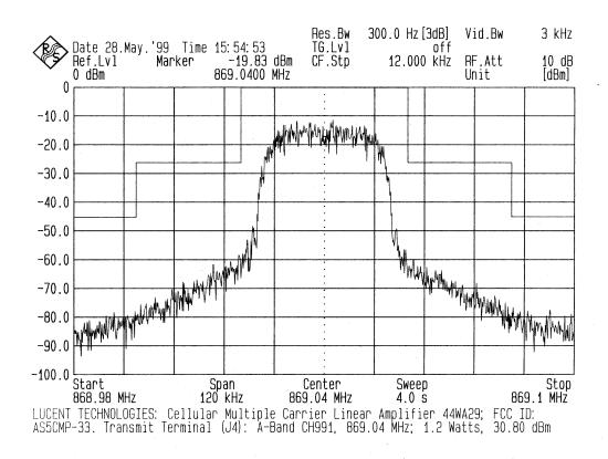
Cellular A-Band Channel 991 869.04 MHz Cellular TDMA Multi Carrier Linear Amplifier, 44WA29, output at transmit antenna terminal
