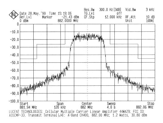
Cellular A-Band Channel 400, 882.00 MHz Cellular TDMA Multi Carrier Linear Amplifier, 44WA29, output at transmit antenna terminal
