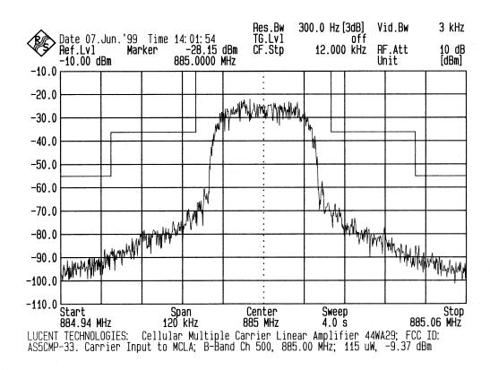
Cellular B-Band Channel 500, 885.00 MHz Cellular TDMA Multi Carrier Linear Amplifier, 44WA29, input signal to CMCLA
