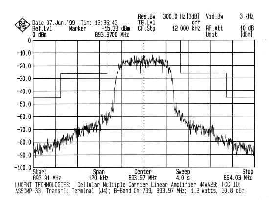
Cellular B-Band Channel 799, 893.97 MHz Cellular TDMA Multi Carrier Linear Amplifier, 44WA29, output at transmit antenna terminal
