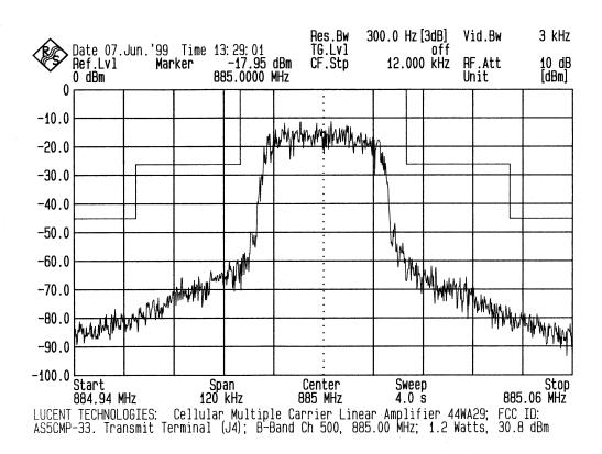
Cellular B-Band Channel 500, 885.00 MHz Cellular TDMA Multi Carrier Linear Amplifier, 44WA29, output at transmit antenna terminal
