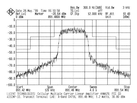
Cellular A-Band Channel 716, 891.48 MHz Cellular TDMA Multi Carrier Linear Amplifier, 44WA29, output at transmit antenna terminal
