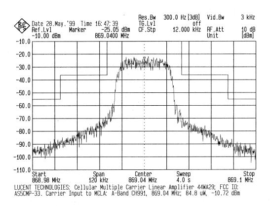
Cellular A-Band Channel 991 869.04 MHz Cellular TDMA Multi Carrier Linear Amplifier, 44WA29, input signal to CMCLA
