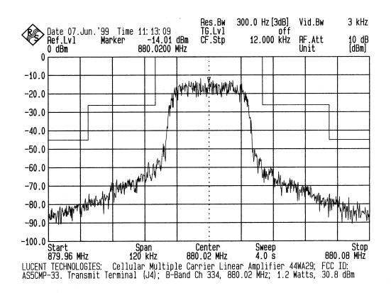
Cellular B-Band Channel 334, 880.02 MHz Cellular TDMA Multi Carrier Linear Amplifier, 44WA29, output at transmit antenna terminal
