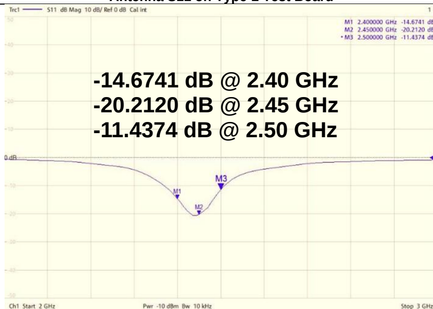
Antenna VSWR on Type-2 Test Board
