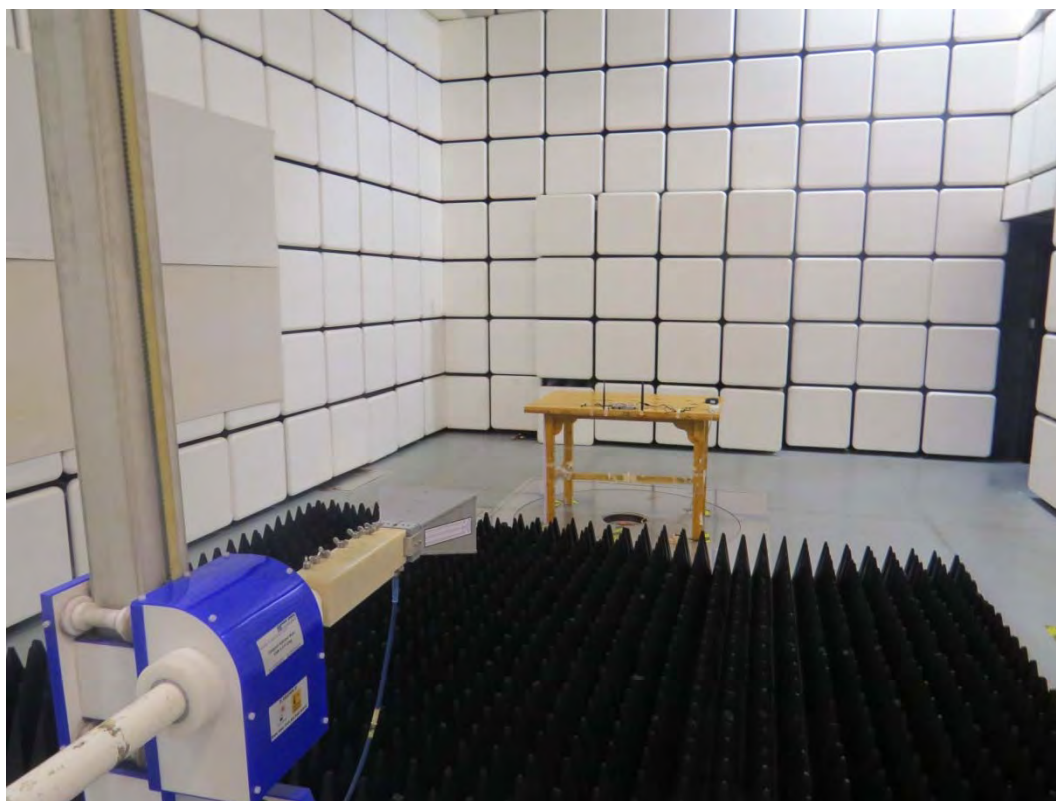
Picture 2: Radiated Spurious Emissions Test setup
