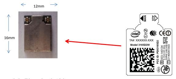
Label will be replaced with laser etching on the metal shield for high volume manufacturing.
