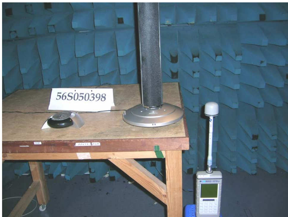
Maximum Permissible Exposure Measurement Test Setup (Rear Round Speaker)
