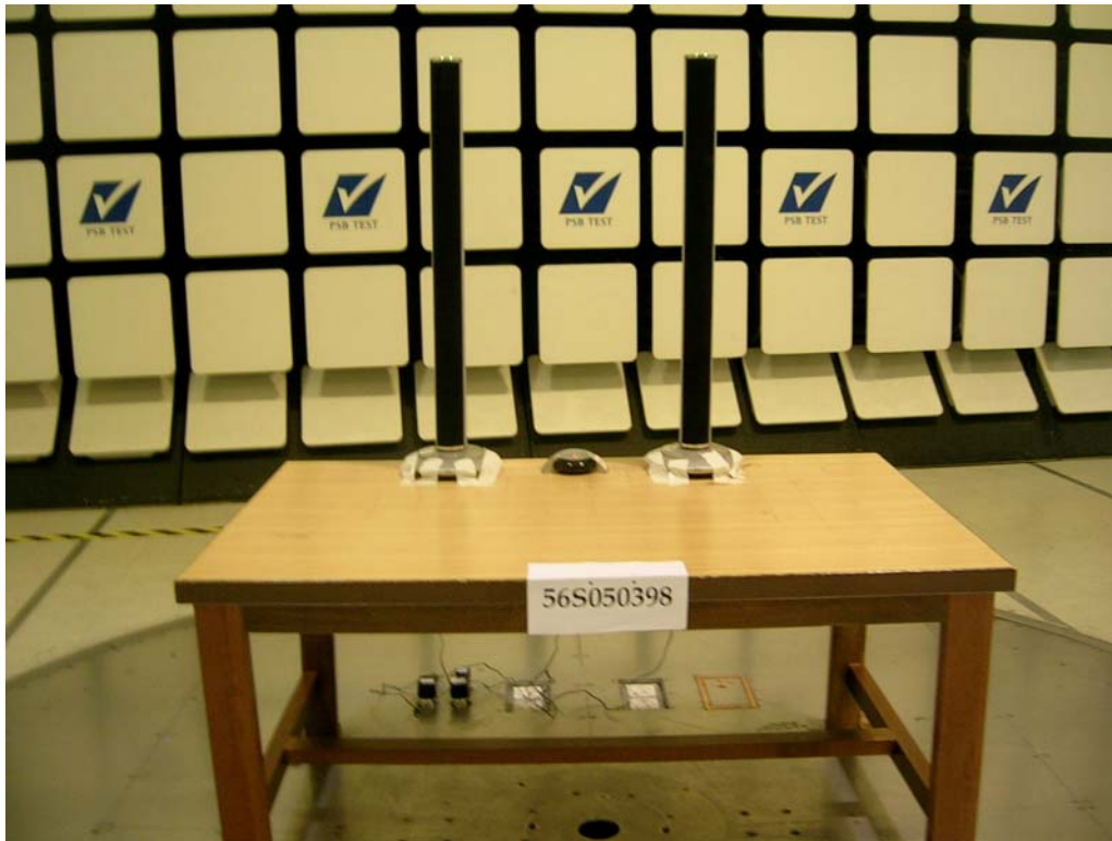
Radiated Emissions Setup (Front View)
