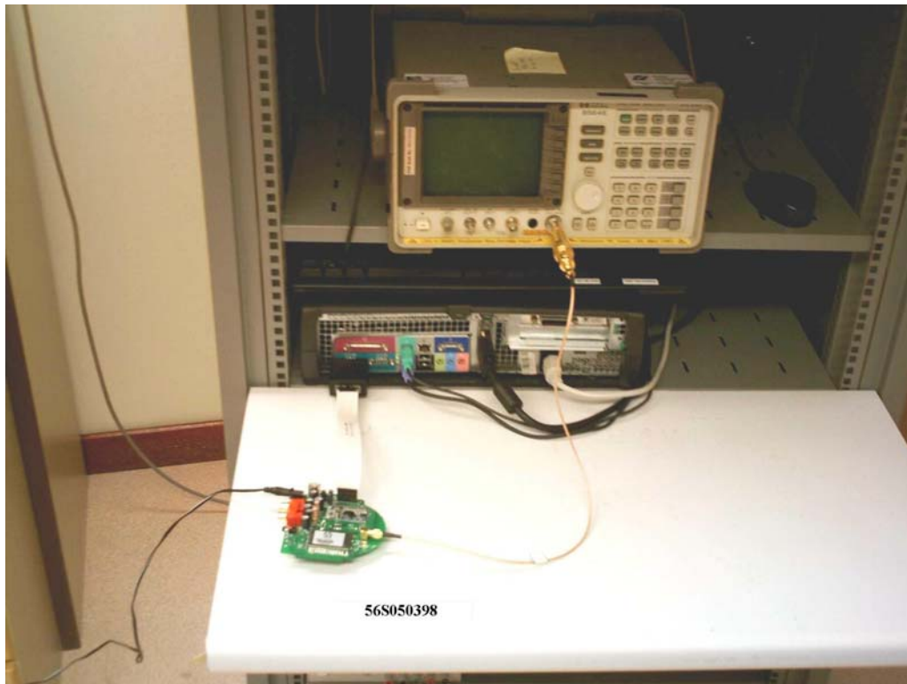
Carrier Frequency Separation Measurement Test Setup
