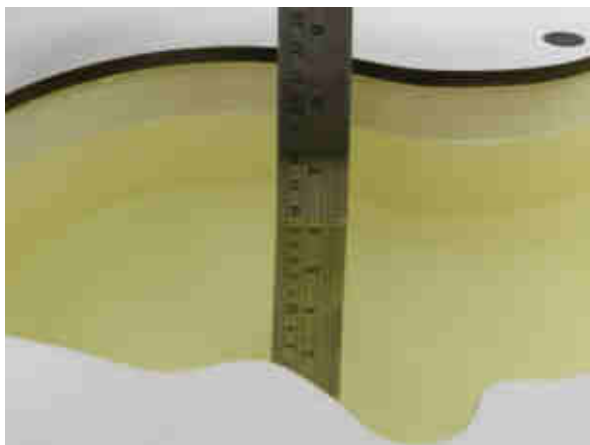
Fig 10.1 Photo of Liquid Height for Head SAR
