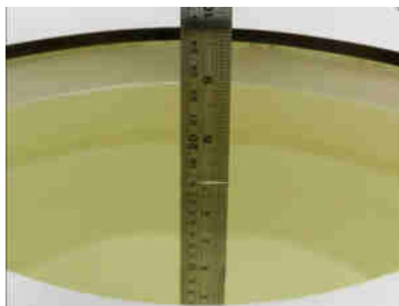
Fig 10.2 Photo of Liquid Height for Body SAR
