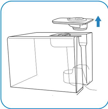
2. Lift up the water tank to remove.
