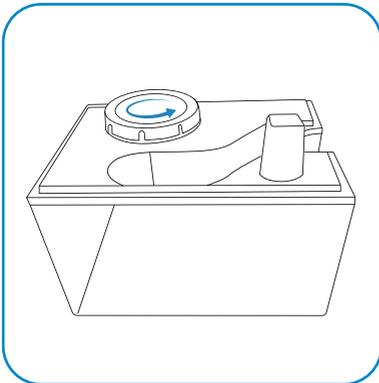
3. Flip the water tank upside down and twist the cap counterclockwise to open the tank.
