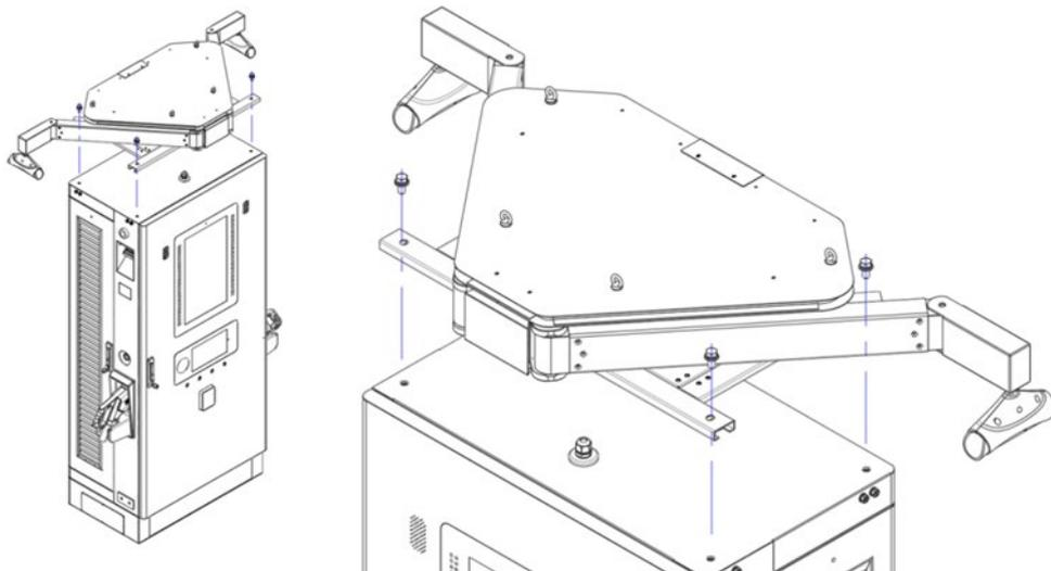
1. Use the cardan shaft fixing bracket to fix the cardan shaft to the short shaft of the cable management system.
