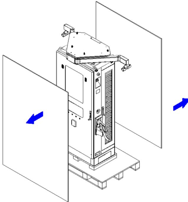
Figure 16. Remove the Front and Back Boards
