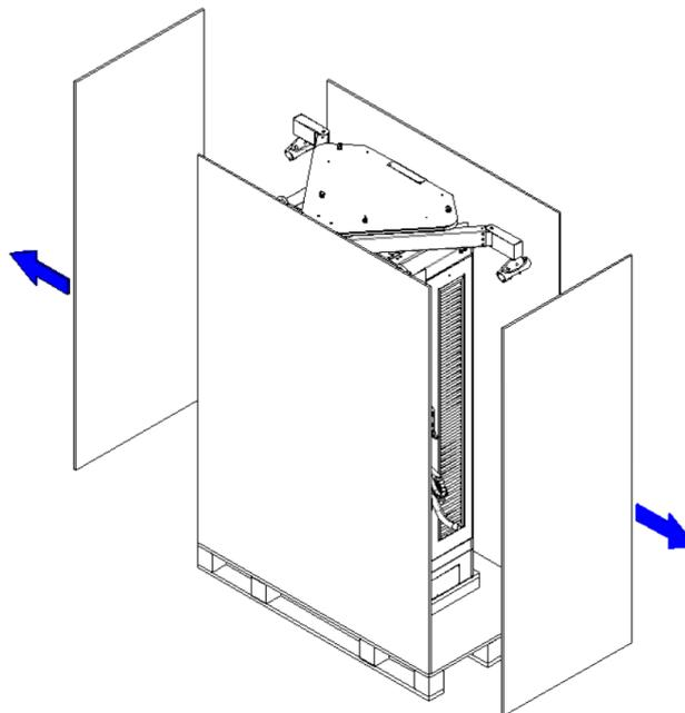
Figure 15. Remove the Left and Right Side Boards.
