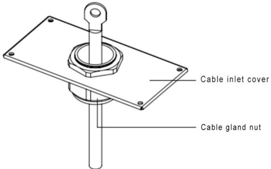
4. Assemble the cable inlet cover nut with a socket spanner or ratchet wrench.
