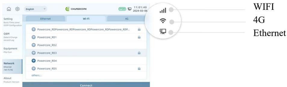
Figure 38. Network Configuration Signal Icon
