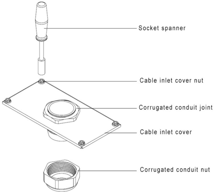
2. Thread the cable into the corrugated conduit nut and corrugated conduit joint in turn.
