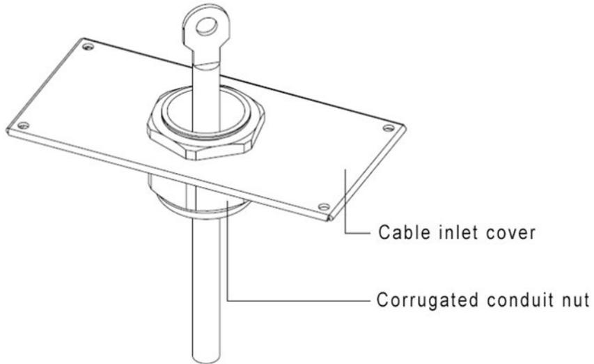
4. After assembling the cable inlet cover nut with a socket spanner or ratchet wrench, seal the cable inlet with fireproofing mud.
