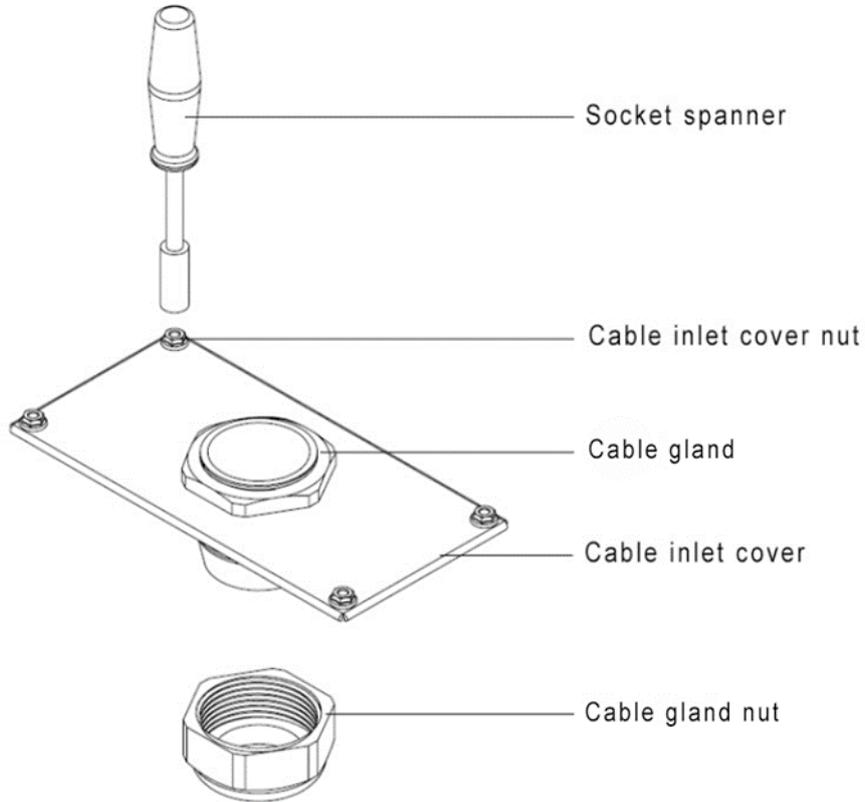
2. Thread the cable into the cable gland nut and cable gland in turn.
