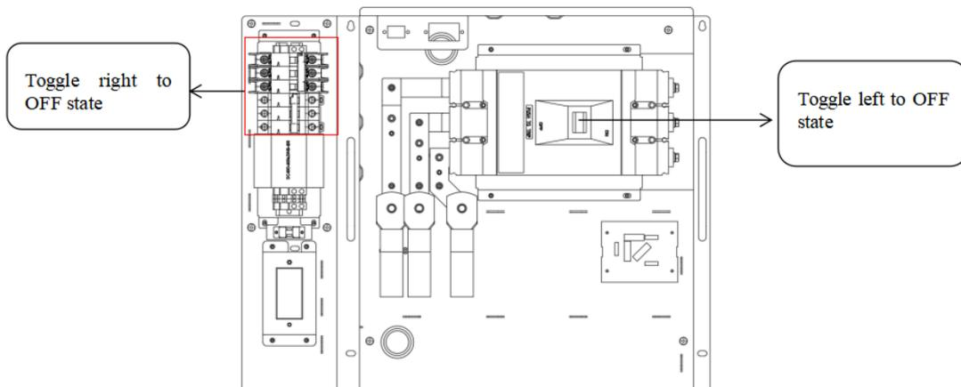
Figure 55. Turning Off the Circuit Breaker, leakage Protection and Air Switch
