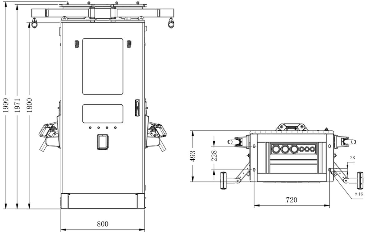
Figure 9. Installation Size
