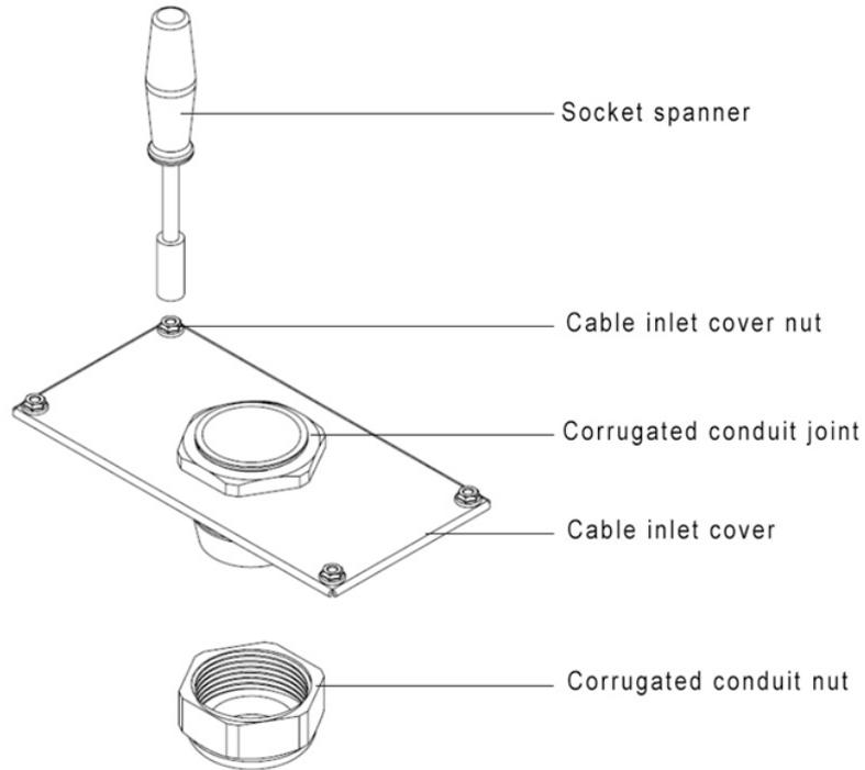
2. Thread the corrugated conduit and cable into the corrugated conduit nut and corrugated conduit joint in turn.
