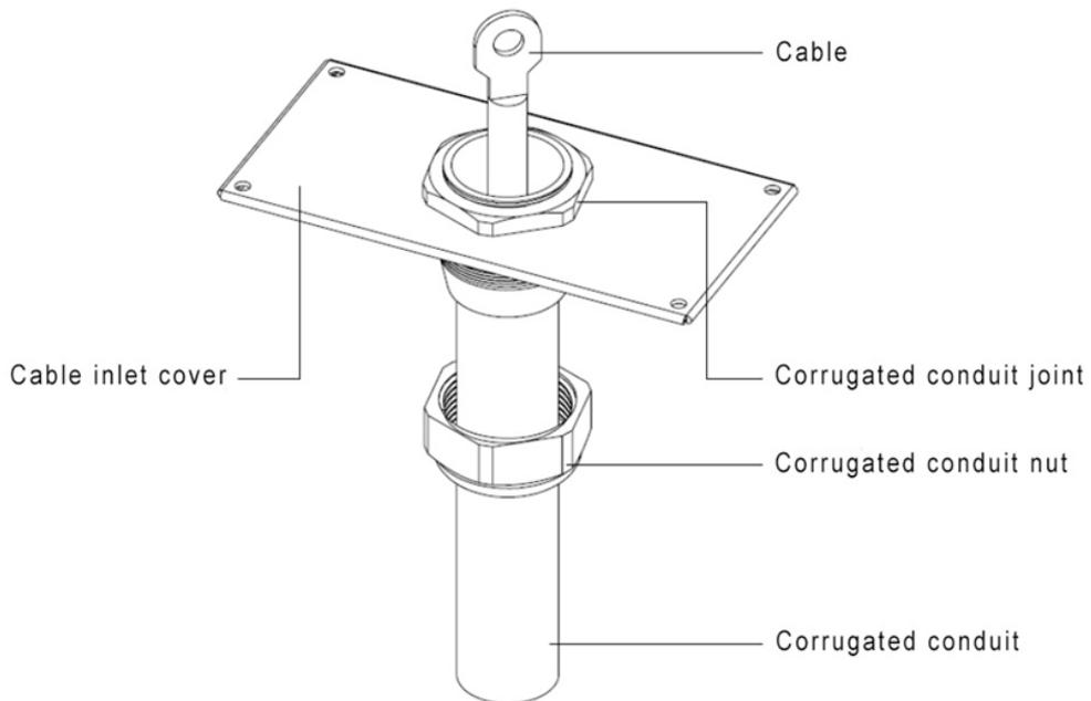
3. After tightening the corrugated conduit nuts, place the cable inlet cover plate back to the bottom of the EVSE.
