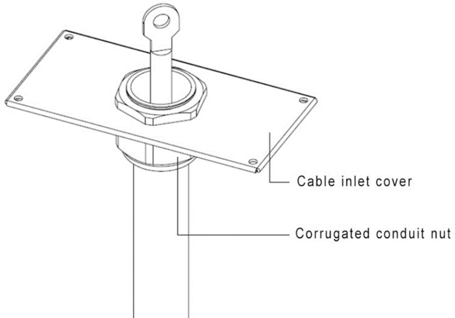
4. Assemble the cable inlet cover nut with a socket spanner or ratchet wrench.
