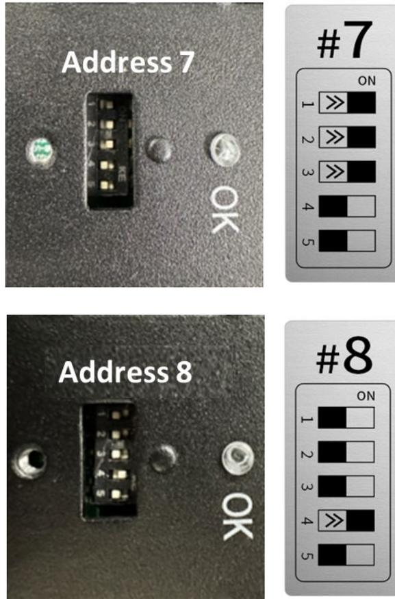
Figure 29. Power Module Addresses for Eight ACE Power Modules
