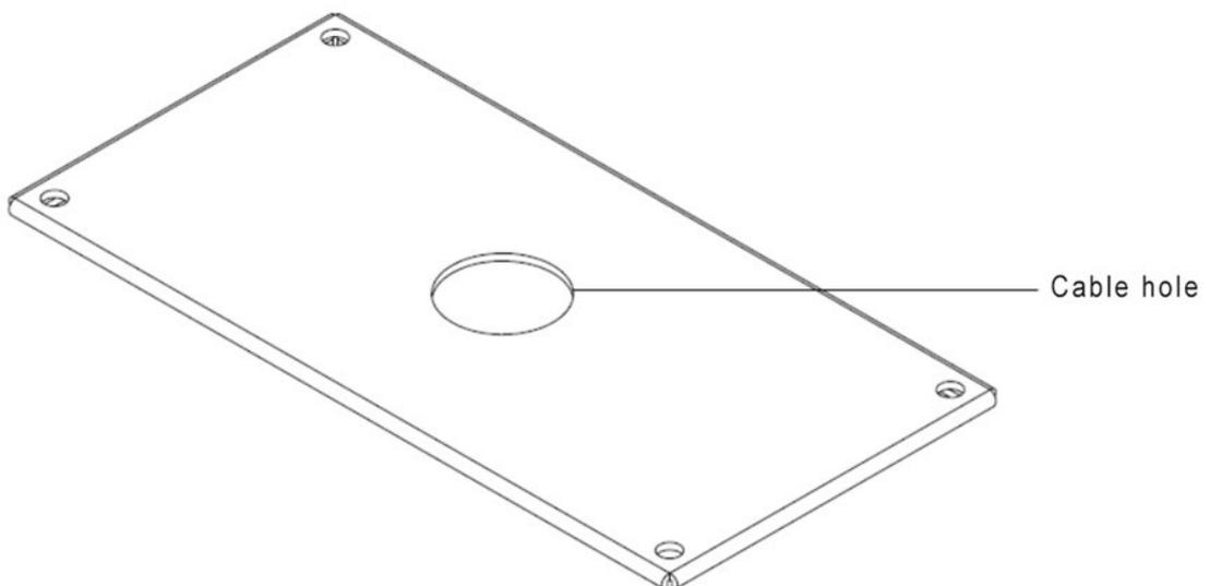
3. After threading the cable into the cable hole, place the cable inlet cover plate back to the bottom of the EVSE.
