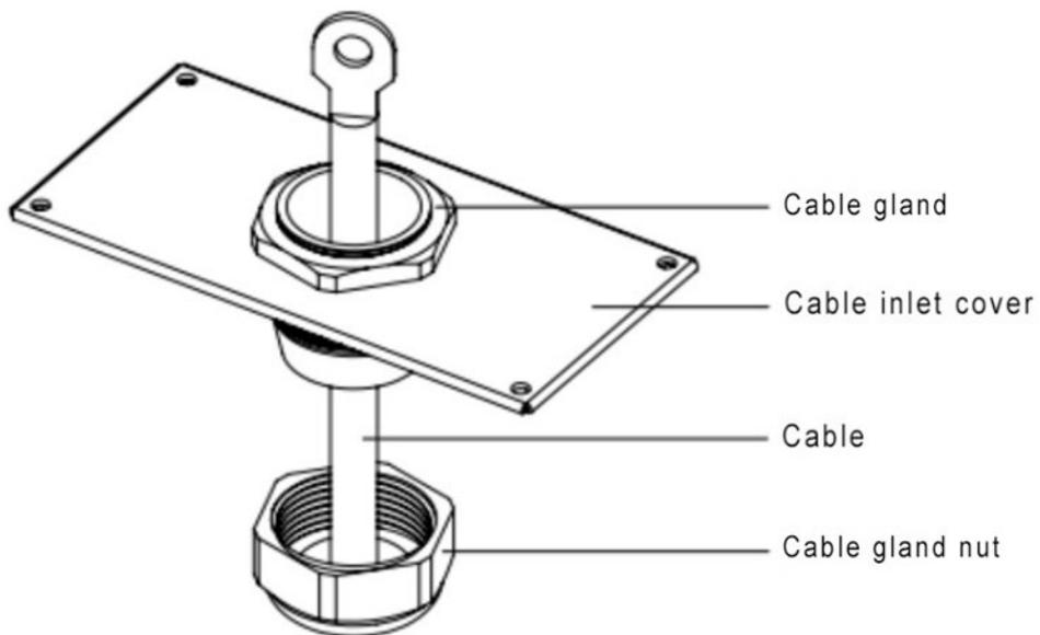
3. After tightening the cable gland nut, place the cable inlet cover back to the bottom of the EVSE.
