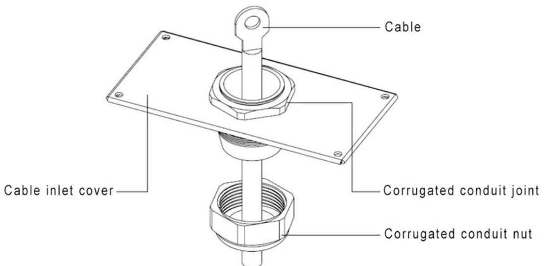
3. After tightening the corrugated conduit nuts, place the cable inlet cover plate back to the bottom of the EVSE.
