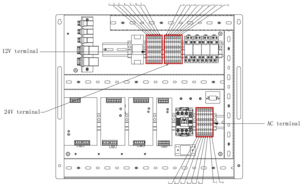
Figure 24. Terminal Points to Check for Short Circuit
