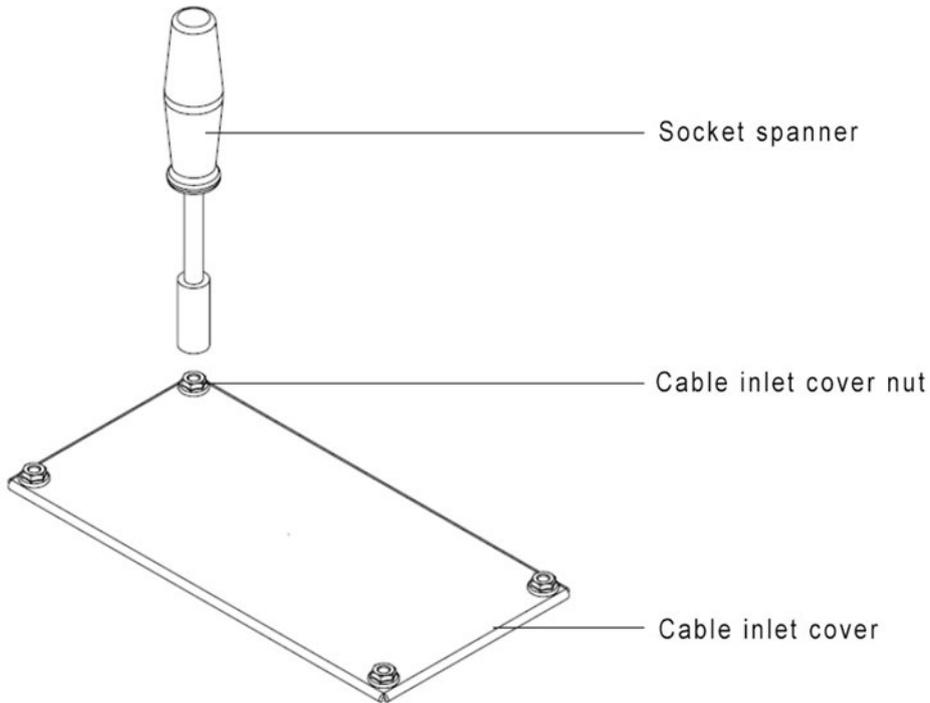
2. According to the equipped inlet cable diameter, the customer can drill the corresponding size of the cable hole.
