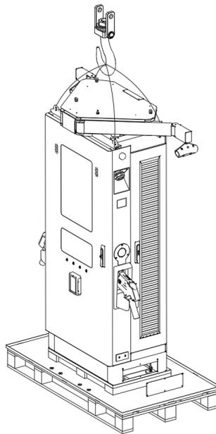
Figure 19. Lifting the EVSE with a Crane
