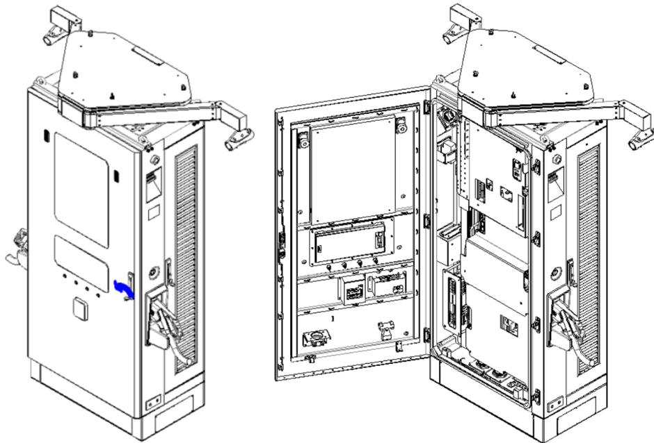
Figure 54. Open the EVSE Front Door
