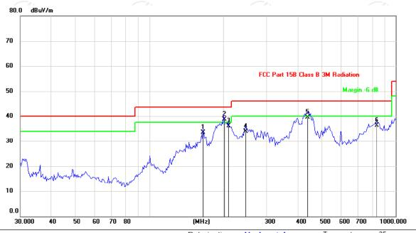
Site Polarization: Horizontal Temperature: 25 Minit: FCC Part 15B Class B 3M Radiation Power: AC 120V/60Hz Humidity: 55 %
