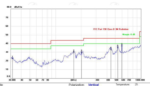
Limit: FCC Part 15B Class B 3M Radiation Power: AC 120V/60Hz
